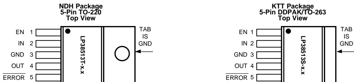
Pin Functions for TO-220 and DDPAK/TO-263 Packages
