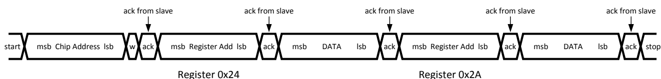
Figure 23. Multi-Byte I 2 C Command
