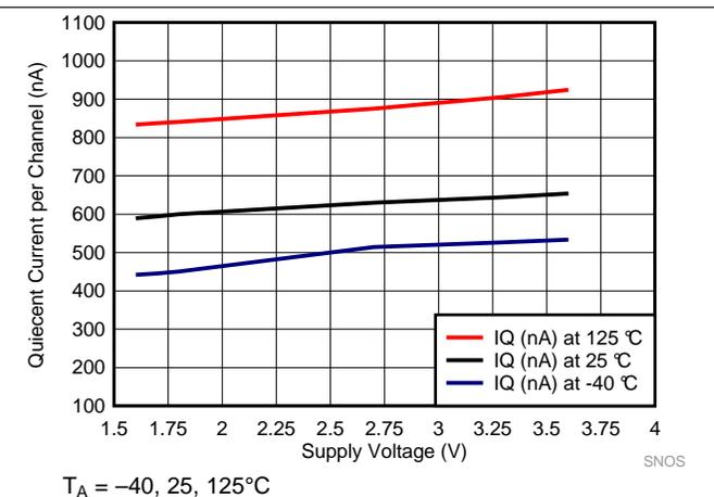
Figure 24. Per Channel Quiescent Current vs Supply Voltage
