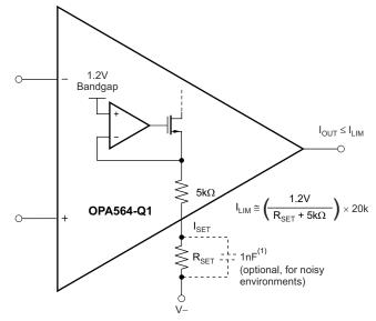
1. At power-on, this capacitor is not charged. Therefore, the OPA564-Q1 is programmed for maximum output current. Capacitor values > 1nF are not recommended.
