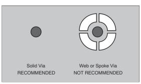
Figure 8-16. Via Connection Methods
