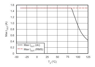
Figure 7-8. Maximum Output Current vs Junction Temperature
