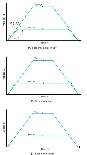
(1) The power-supply sequence illustrated in (A) is not allowed because this power-supply sequence damages the device.
