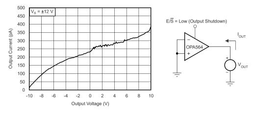
Figure 7-6. Output Shutdown Output Impedance
