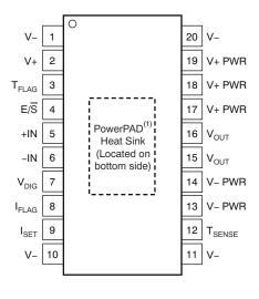
(1) PowerPAD is internally connected to V-, Soldering the PowerPAD to the PCB is always required, even with applications that have low power dissipation.
