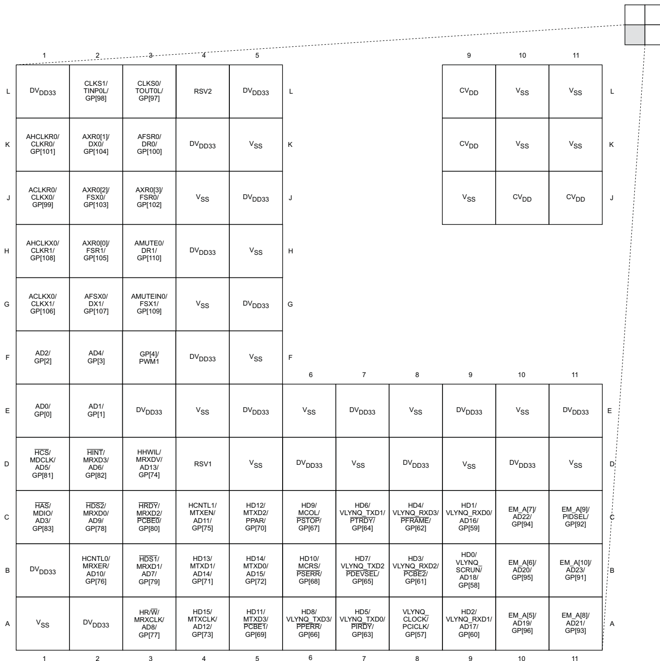
Figure 2-9. GDU Pin Map [Quadrant D]
