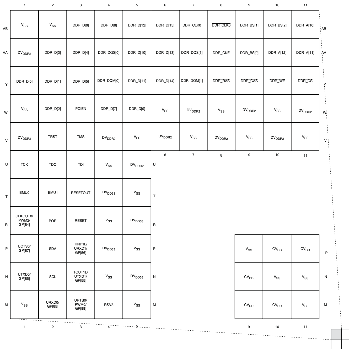
Figure 2-6. GDU Pin Map [Quadrant A]
