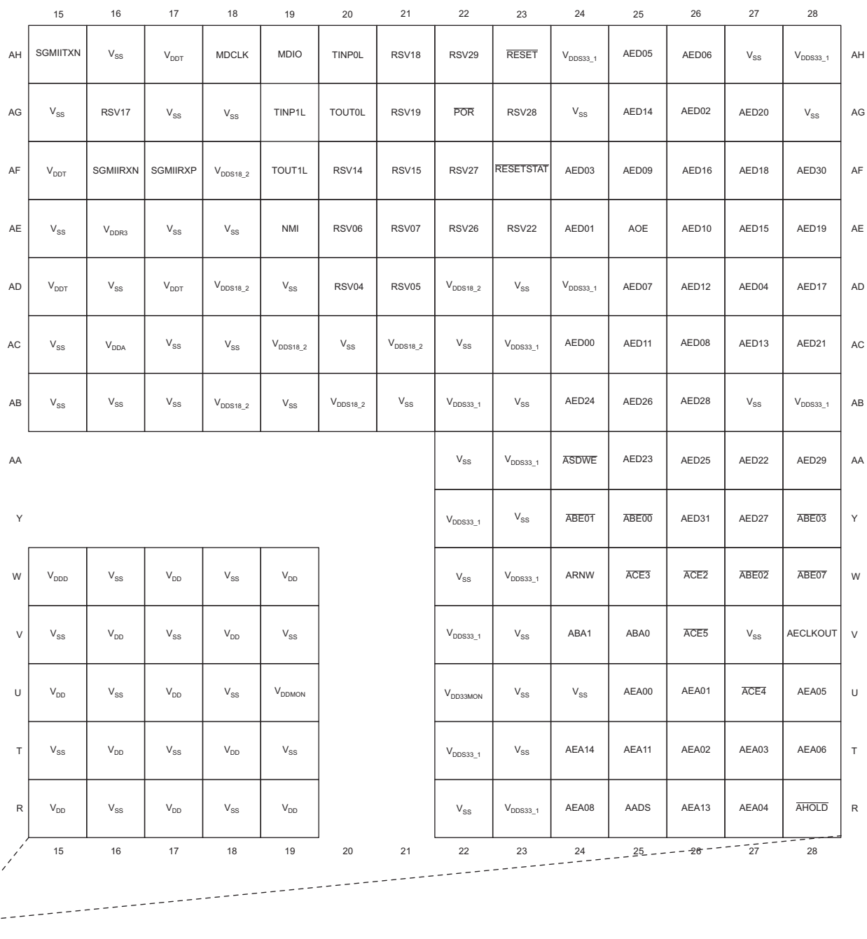
Figure 3-3. TCI648F Pin Map (Bottom View) [Quadrant B]
