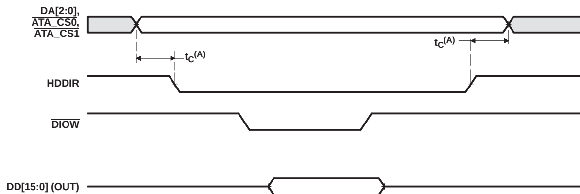
Figure 6-38. ATA/CF HDDIR Taskfile Write/Single PIO Write Timing
