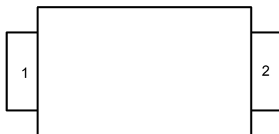
Figure 4-1. DYP Package, 2-Pin SMAF (Top View)
