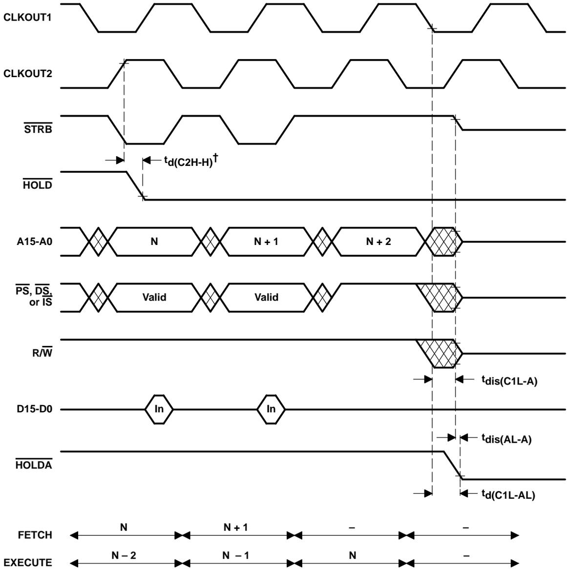
† HOLD is an asynchronous input and can occur at any time during a clock cycle. If the specified timing is met, the exact sequence shown occurs; otherwise, a delay of one CLKOUT2 cycle occurs.
