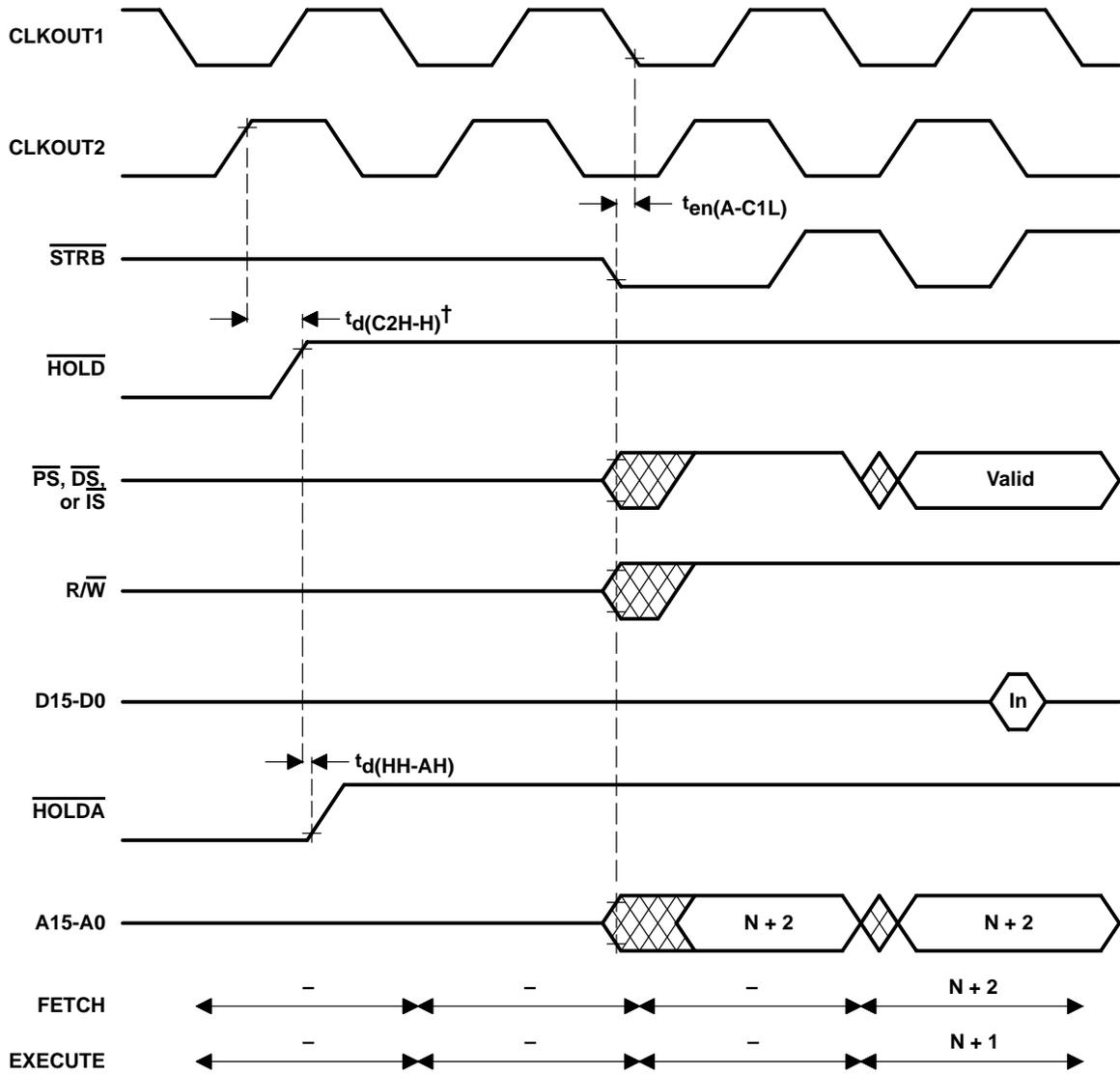
$^\dagger$   $\overline{\text{HOLD}}$  is an asynchronous input and can occur at any time during a clock cycle. If the specified timing is met, the exact sequence shown occurs; otherwise, a delay of one CLKOUT2 cycle occurs.
