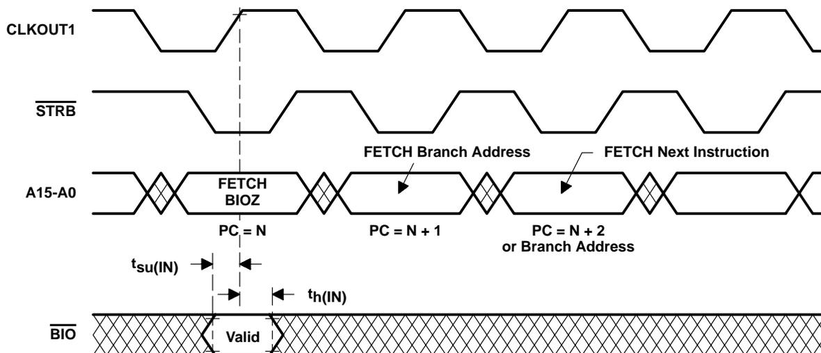
Figure 11.  $\overline{BIO}$  Timing
