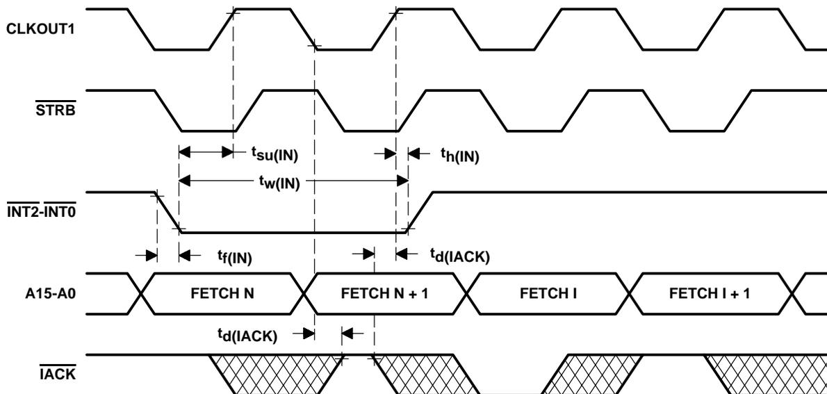
Figure 10. Interrupt Timing
