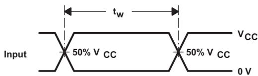
**Figure 6-3. Voltage Waveforms Pulse Duration**
