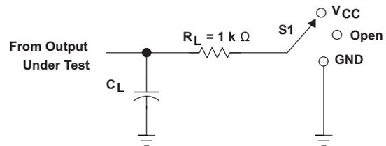
**Figure 6-2. Load Circuit For 3-State and Open-Drain Outputs**
