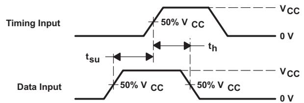
**Figure 6-4. Voltage Waveforms Setup and Hold Times**
