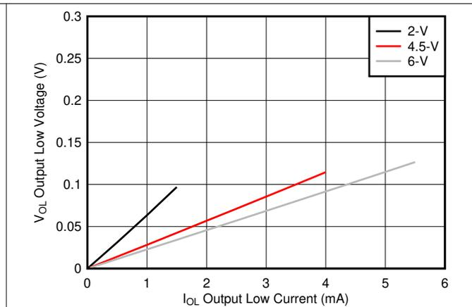
Figure 6-2. Typical output voltage in the low state (V<sub>OL</sub>)
