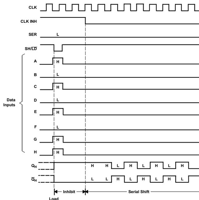
Figure 4. Typical Shift, Load, and Inhibit Sequence
