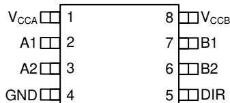
Figure 4-1. DCT Package, 8-Pin SSOP (Top View)
