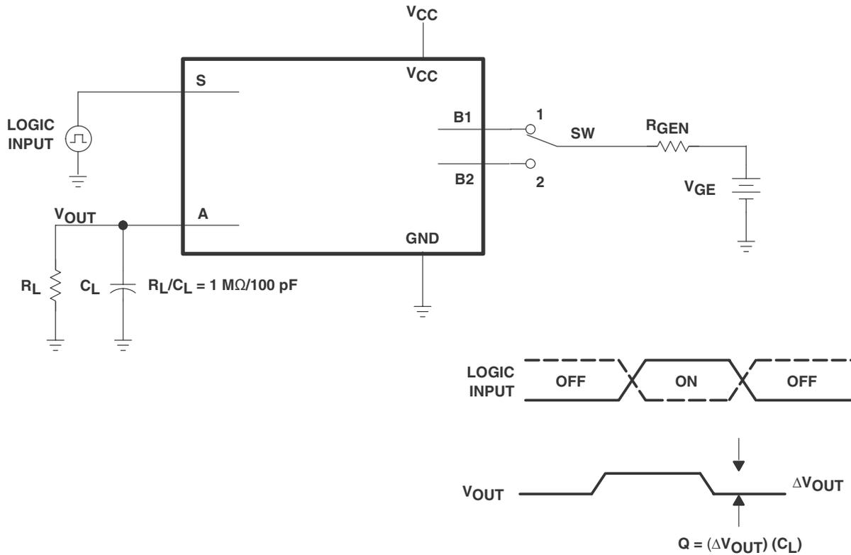
Figure 6-8. Charge-Injection Test
