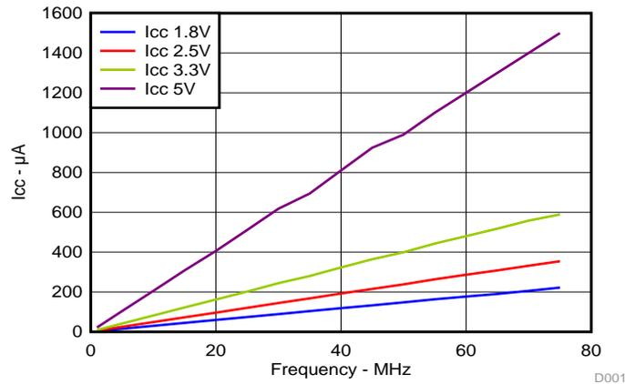
**Figure 6. I<sub>CC</sub> vs Frequency**
