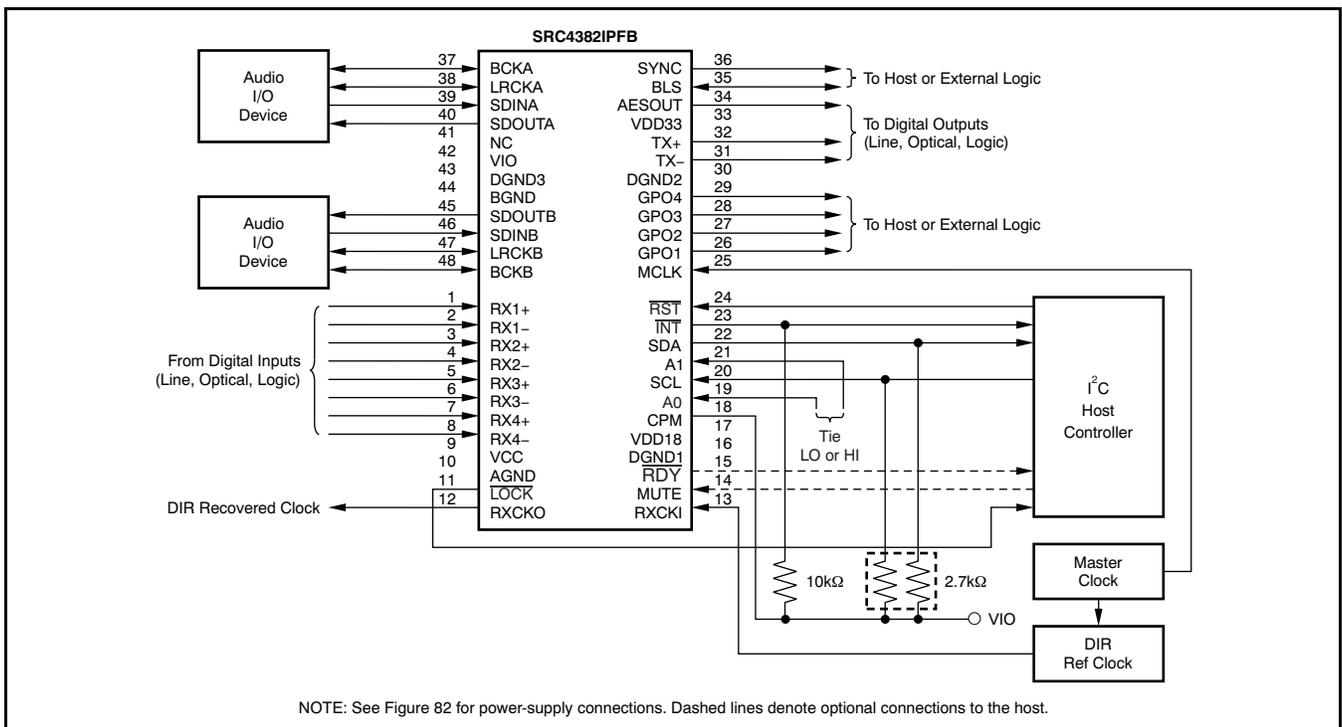
**Figure 81. Typical Application Diagram Using I²C Host Interface**
