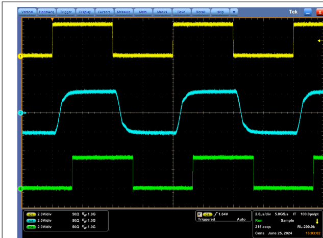
Ch 1: D Input, Ch2: V A Ch3: V B Ch4: R V CC = 3.3V Output Data rate: 20Mbps
