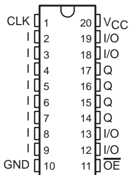
TIBPAL16R4' C SUFFIX ... J OR N PACKAGE M SUFFIX ... J OR W PACKAGE (TOP VIEW)
