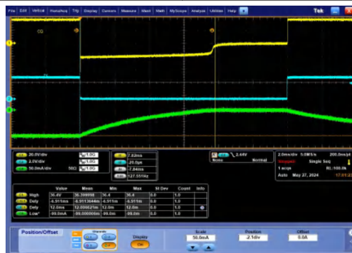
Figure 9-5. CQ Power Up Delay, t_{UVLO} (Pin mode or the default 00b setting in SPI mode)
