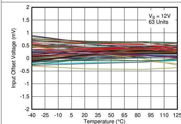
Figure 5-17. Input Offset Voltage vs. Temperature at 12V
