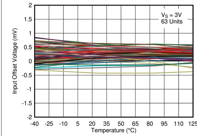
Figure 5-15. Input Offset Voltage vs. Temperature at 3V
