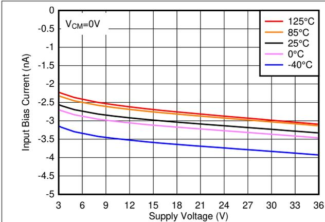
Figure 5-7. Input Bias Current vs. Supply Voltage
