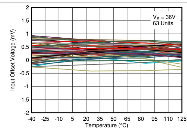
Figure 5-18. Input Offset Voltage vs. Temperature at 36V
