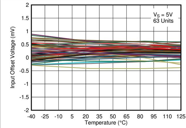
Figure 5-16. Input Offset Voltage vs. Temperature at 5V
