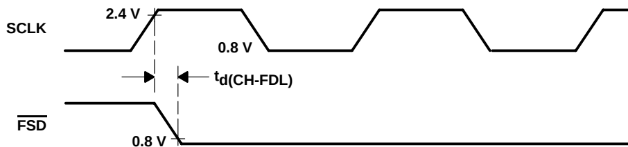
Figure 4 – 6. Slave SCLK to \overline{\text{FSD}} Timing
