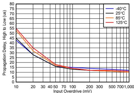
Figure 3-1. Prop Delay, High to Low, 12V
