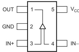
Figure 5-1. TLV3701 DBV Package 5-Pin SOT-23 Top View
