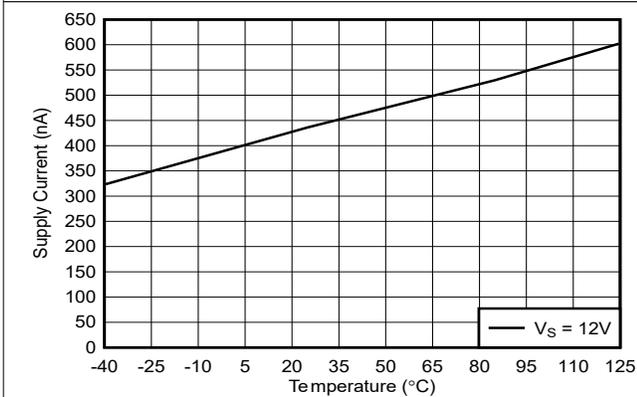
**Figure 6-11. Supply Current vs. Temperature (Output High), Push-Pull**
