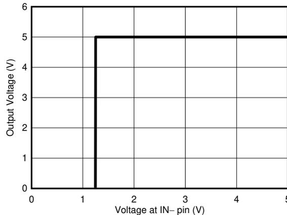
Figure 8-2. Transfer Function for the Threshold Detector
