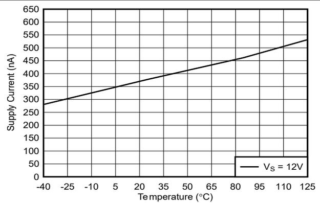
**Figure 6-10. Supply Current vs. Temperature (Output Low), Push-Pull**
