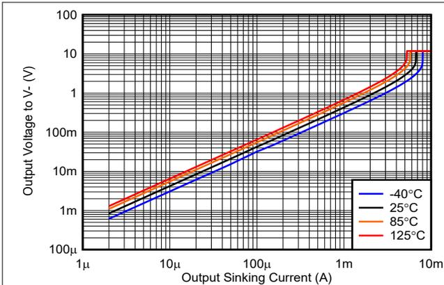
**Figure 6-7. Output Voltage vs. Output Sinking Current, 12V**
