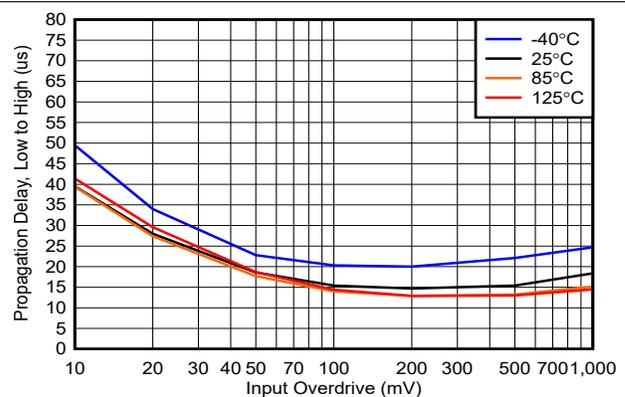
**Figure 6-12. Propagation Delay, Low to High, 12V, Push-Pull**
