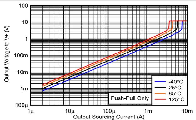
Figure 6-6. Output Voltage vs. Output Sourcing Current, 12V
