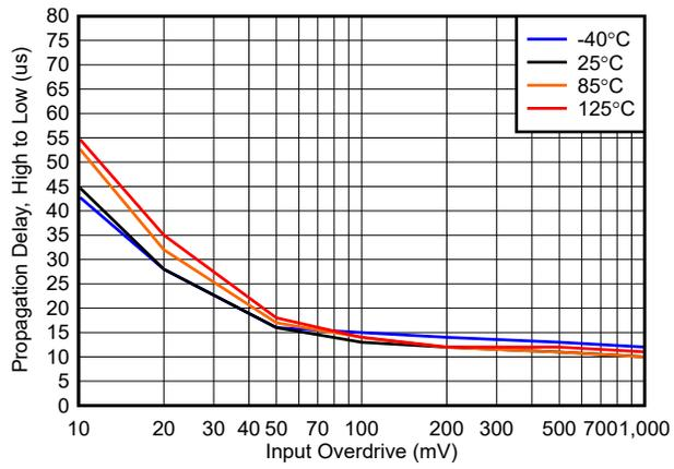
Figure 6-13. Propagation Delay, High to Low, 12V
