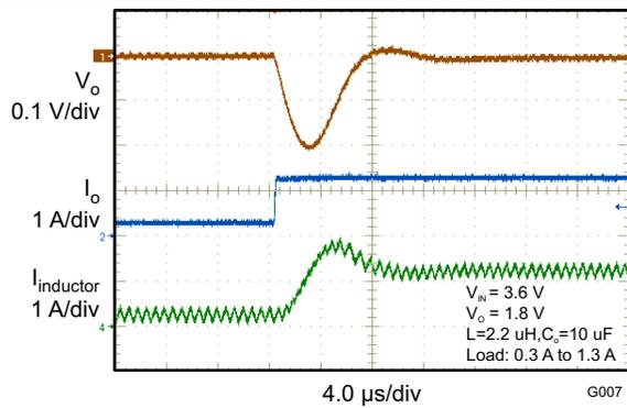
Figure 17. Load Transient
