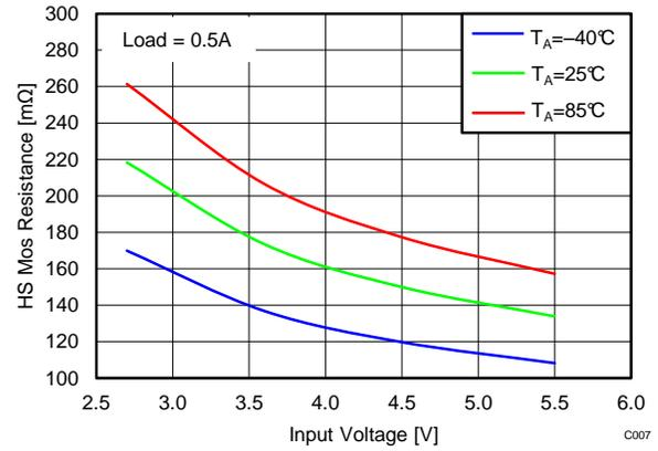
Figure 2. High-Side FET R<sub>DS(on)</sub> vs Input Voltage
