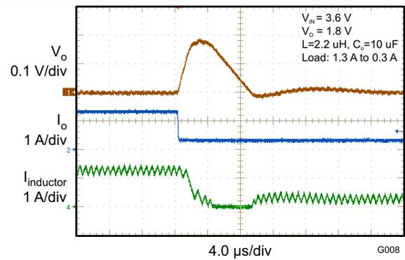
Figure 18. Load Transient
