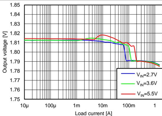
Figure 13. Output Voltage vs Load Current
