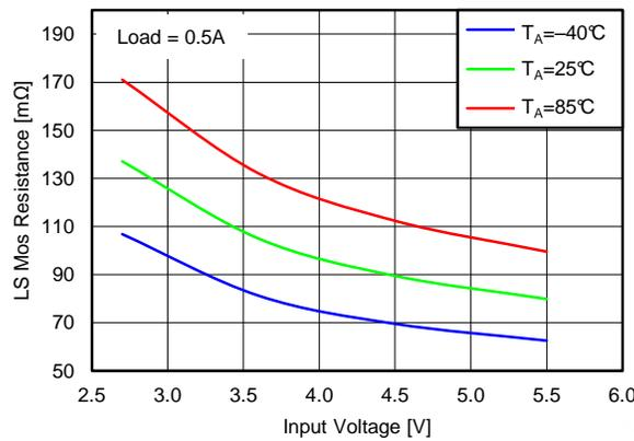
Figure 3. Low-Side FET R<sub>DS(on)</sub> vs Input Voltage
