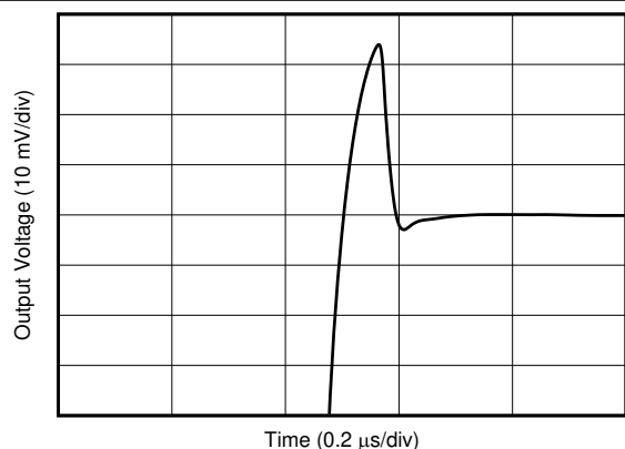
Figure 7-31. Small-Signal Step Response
