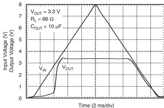
**Figure 6-23. Power-Up, Power-Down for Legacy Chip**
