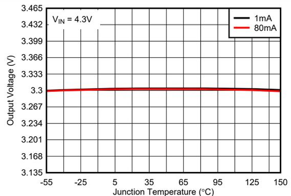
Figure 6-6. Output Voltage vs Junction Temperature for New Chip
