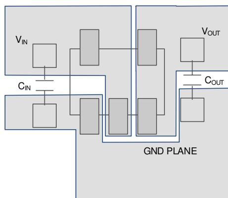
**Figure 8-11. Layout Example for the DBV Package**
