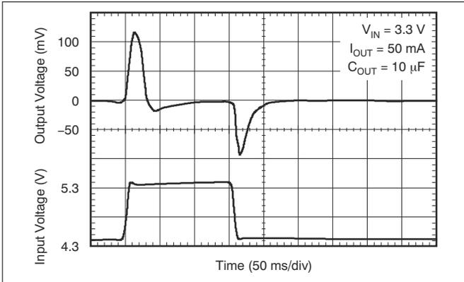
Figure 6-25. Line Transient Response for Legacy Chip
