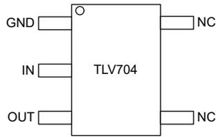
**Figure 5-1. DBV Package, 5-Pin SOT-23 (Top View)**
