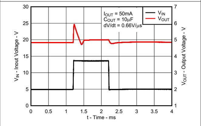
Figure 6-30. Dropout Exit Transient Response for New Chip
