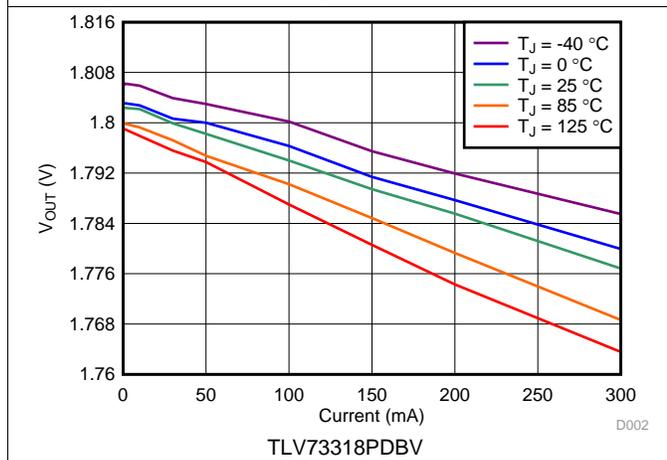
Figure 3. 1.8-V Load Regulation vs  $I_O$  and Temperature
