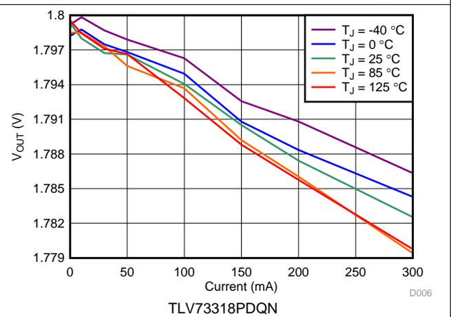
Figure 4. 1.8-V Load Regulation vs  $I_{OUT}$  and Temperature
