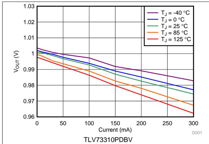
Figure 1. 1.0-V Load Regulation vs  $I_{OUT}$  and Temperature
