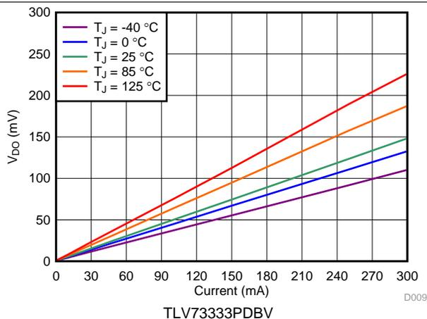
Figure 11. 3.3-V Dropout Voltage vs  $I_{OUT}$  and Temperature
