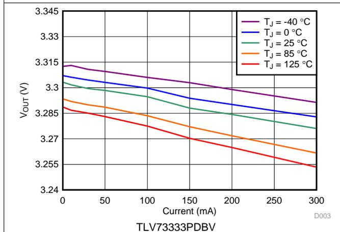
Figure 5. 3.3-V Load Regulation vs  $I_{OUT}$  and Temperature
