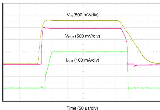
Figure 36. 1.8-V to 1.5-V Regulation at 300 mA
