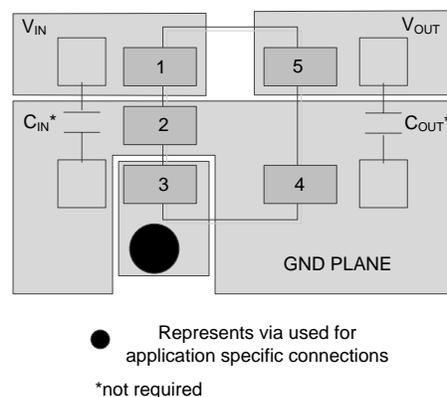
Figure 40. Layout Example for the DBV Package
