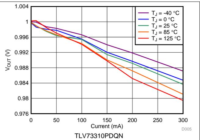
Figure 2. 1.0-V Load Regulation vs  $I_{OUT}$  and Temperature
