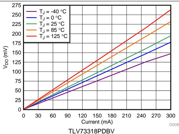
Figure 9. 1.8-V Dropout Voltage vs  $I_{OUT}$  and Temperature
