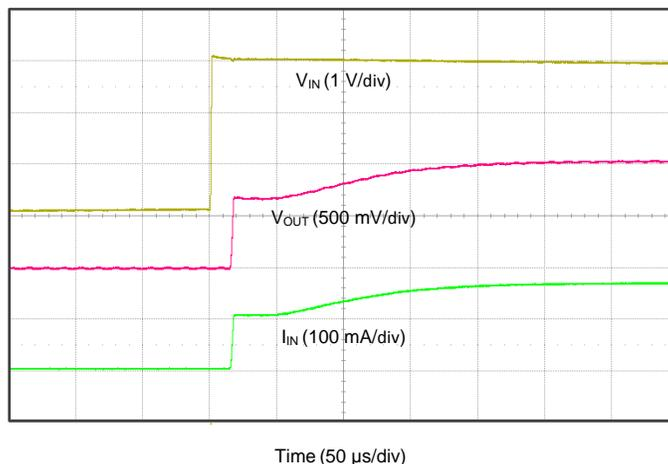
Figure 38. No Inrush Startup, 3.0-V to 1.0-V Regulation
