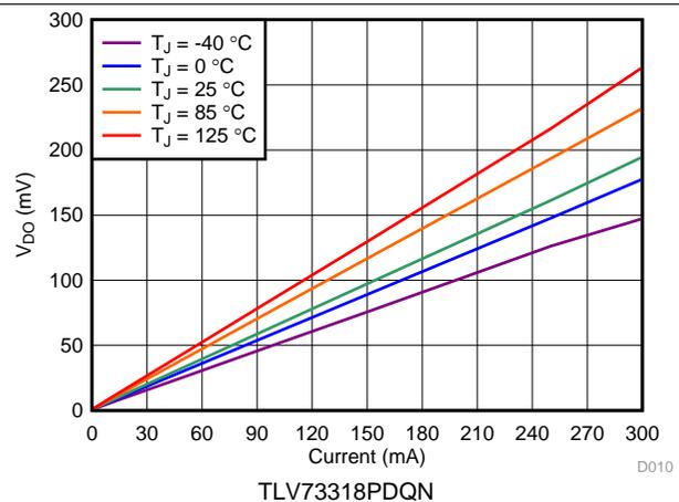
Figure 10. 1.8-V Dropout Voltage vs  $I_{OUT}$  and Temperature
