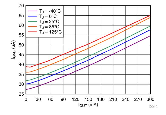
Figure 14. Ground Pin Current vs  $I_{OUT}$  and Temperature
