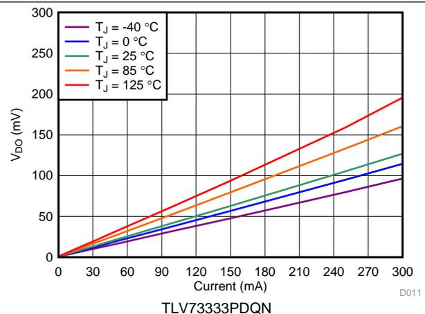
Figure 12. 3.3-V Dropout Voltage vs  $I_{OUT}$  and Temperature
