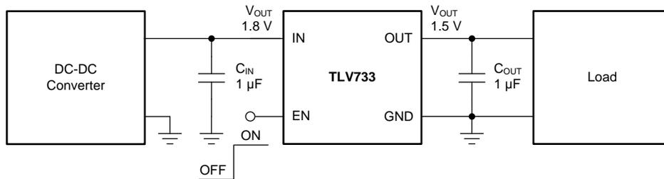
Figure 35. DC-DC Converter Post Regulation
