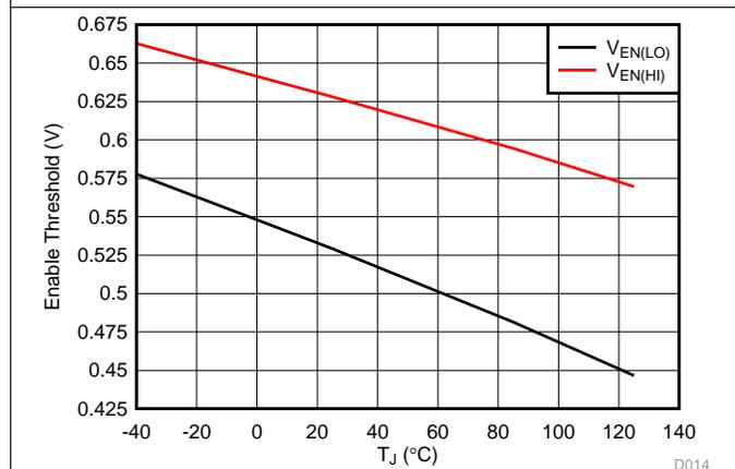
Figure 17. Enable Threshold vs Temperature
