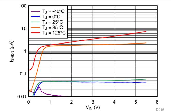
Figure 16. Shutdown Current vs  $V_{IN}$  and Temperature
