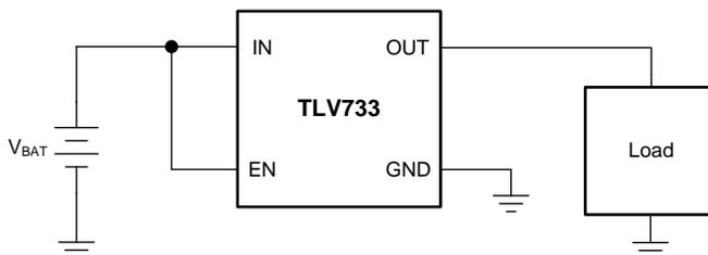
Figure 37. Capacitor-Free Operation from Battery Input Supply
