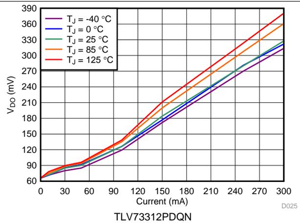
Figure 8. 1.2-V Dropout Voltage vs  $I_{OUT}$  and Temperature
