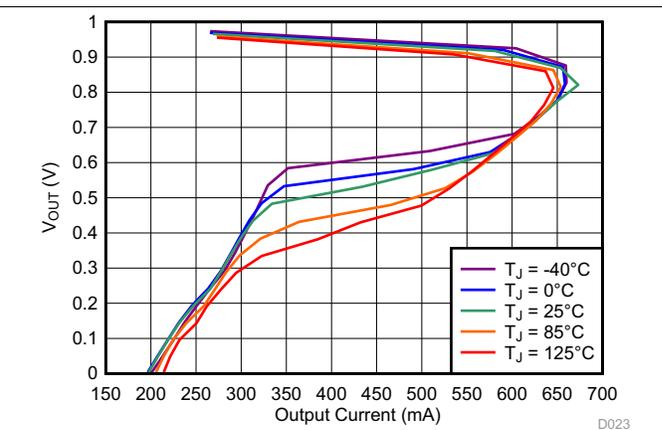
Figure 18. 1.0-V Foldback Current Limit vs  $I_{OUT}$  and Temperature
