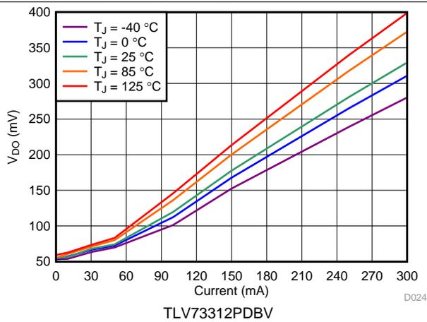
Figure 7. 1.2-V Dropout Voltage vs  $I_{OUT}$  and Temperature
