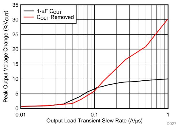
TLV73333PDBV, output current stepped from 50 mA to 300 mA, output voltage change measured at positive  $dl/dt$
