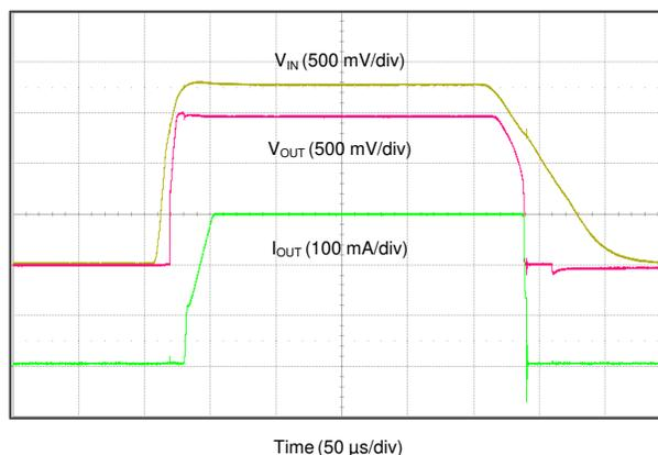
Figure 8-3. 1.8-V to 1.5-V Regulation at 300 mA
