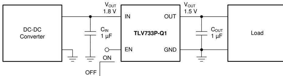
Figure 8-2. DC-DC Converter Post Regulation
