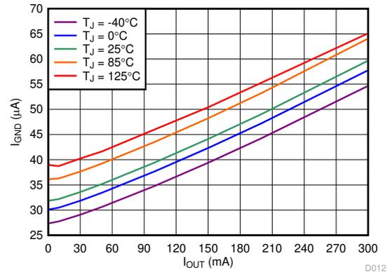
**Figure 6-2. Ground Pin Current vs  $I_{OUT}$  and Temperature**
