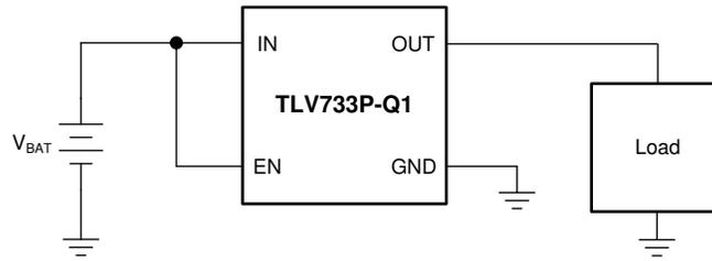
**Figure 8-4. Capacitor-Free Operation from a Battery Input Supply**
