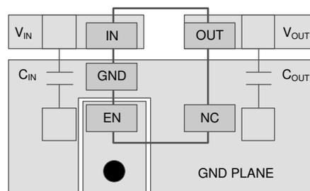
**Figure 7-9. Layout Example for the DBV Package**
