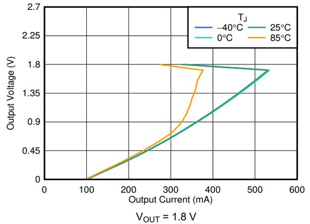
Figure 5-8. Foldback Current Limit vs  $I_{OUT}$
