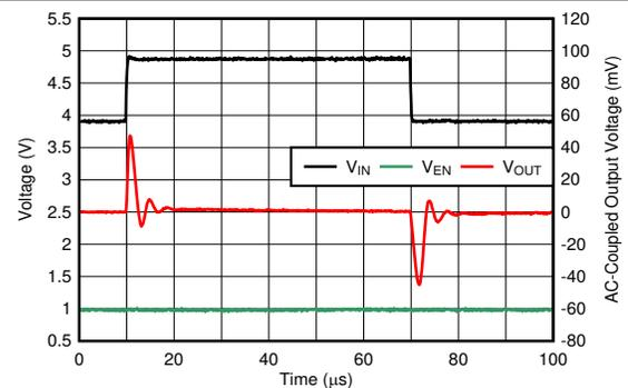
Figure 7-7. VIN Line Transient,  $I_{OUT} = 30$  mA
