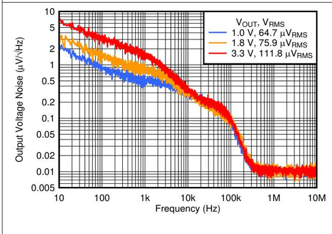
Figure 5-17. Output Noise vs Frequency and  $V_{OUT}$
