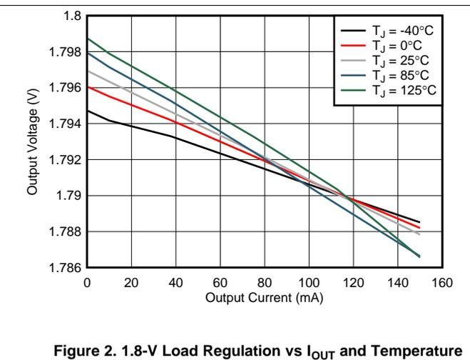
Figure 2. 1.8-V Load Regulation vs  $I_{OUT}$  and Temperature
