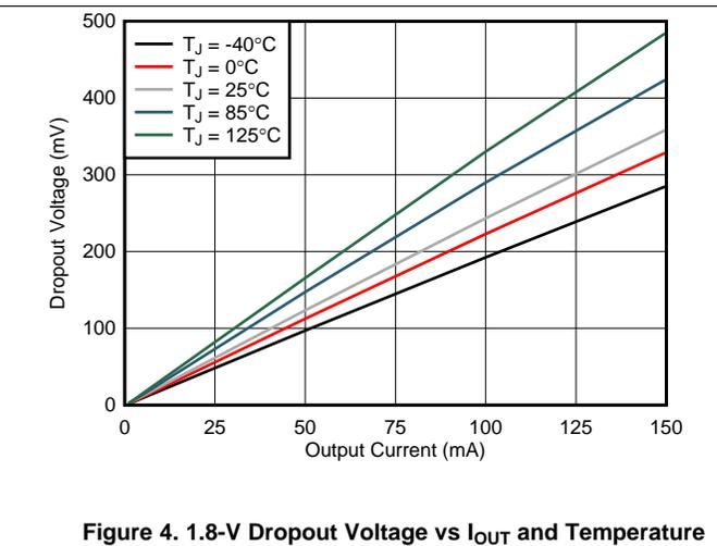
Figure 4. 1.8-V Dropout Voltage vs  $I_{OUT}$  and Temperature
