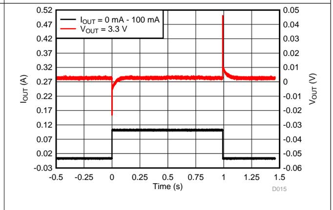
Figure 16. Load Transient
