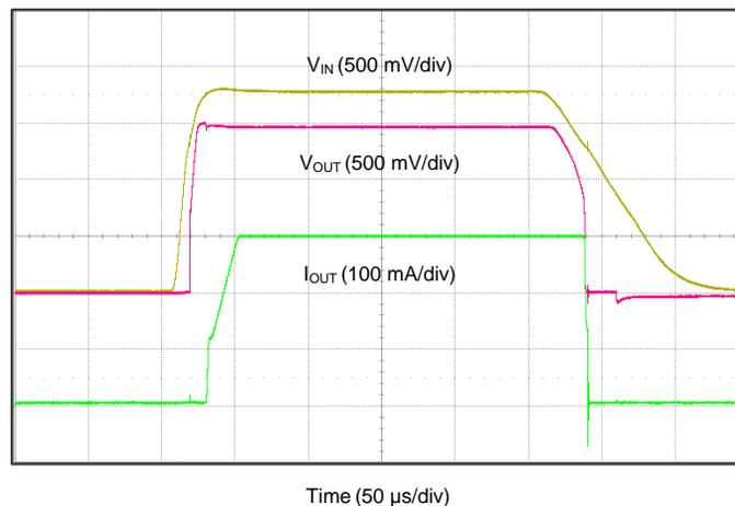
Figure 33. 1.8-V to 1.5-V Regulation at 300 mA
