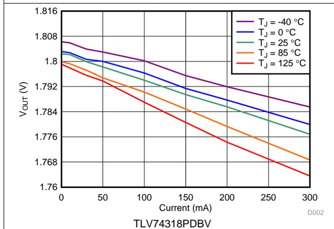
Figure 3. 1.8-V Load Regulation vs  $I_{OUT}$  and Temperature
