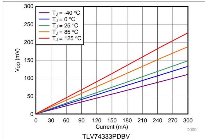
Figure 11. 3.3-V Dropout Voltage vs  $I_{OUT}$  and Temperature
