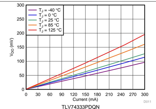
Figure 12. 3.3-V Dropout Voltage vs  $I_{OUT}$  and Temperature
