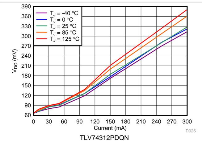
Figure 8. 1.2-V Dropout Voltage vs  $I_{OUT}$  and Temperature
