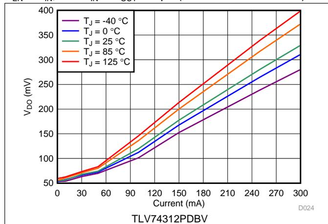
Figure 7. 1.2-V Dropout Voltage vs  $I_{OUT}$  and Temperature
