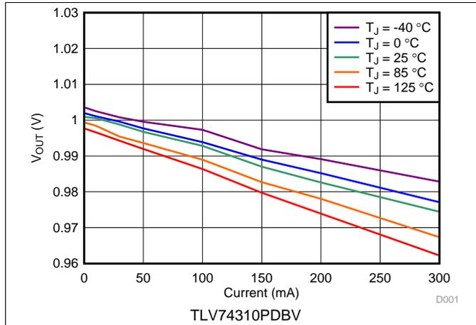
Figure 1. 1-V Load Regulation vs  $I_{OUT}$  and Temperature
