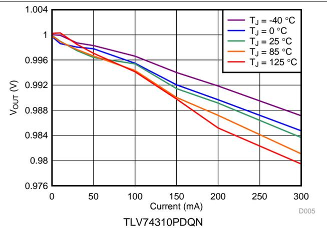
Figure 2. 1-V Load Regulation vs  $I_{OUT}$  and Temperature
