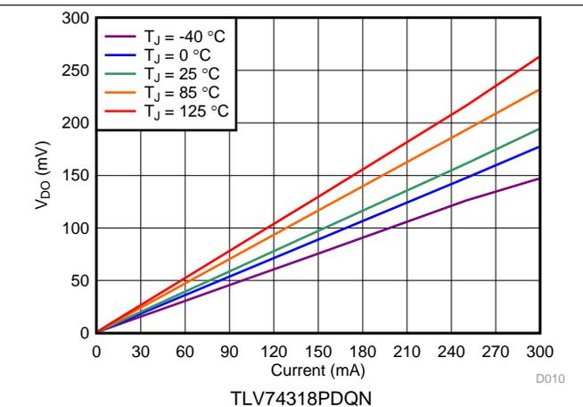
Figure 10. 1.8-V Dropout Voltage vs  $I_{OUT}$  and Temperature
