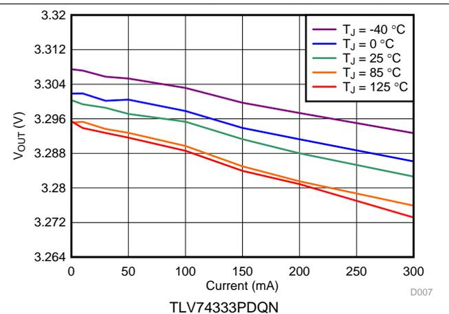
Figure 6. 3.3-V Load Regulation vs  $I_{OUT}$  and Temperature
