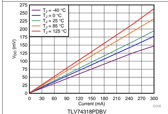
Figure 9. 1.8-V Dropout Voltage vs  $I_{OUT}$  and Temperature
