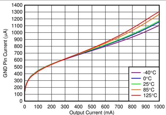
Figure 5-18.  $I_{GND}$  vs  $I_{OUT}$
