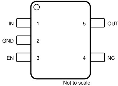
Figure 4-1. DBV Package, 5-Pin SOT-23 (Top View)
