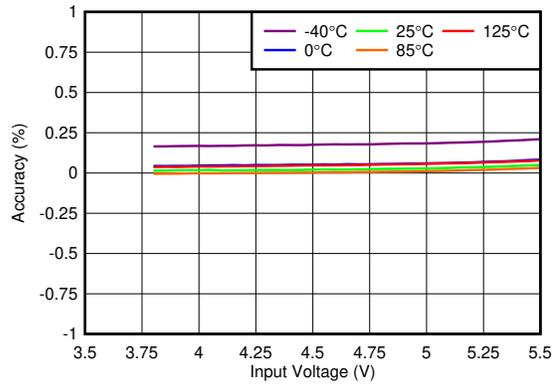
**Figure 5-16. 3.3V Regulation vs  $V_{IN}$  (Line Regulation)**
