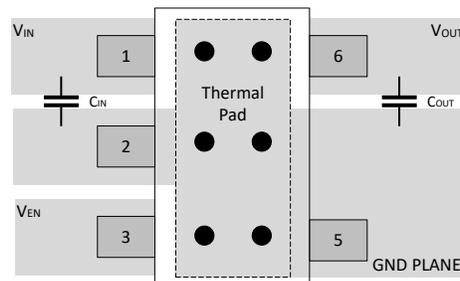
**Figure 7-9. Layout Example: DYD Package**
