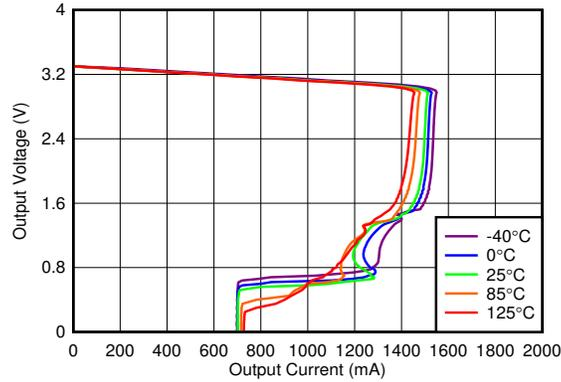
Figure 5-27. 3.3V Foldback Current Limit vs  $I_{OUT}$
