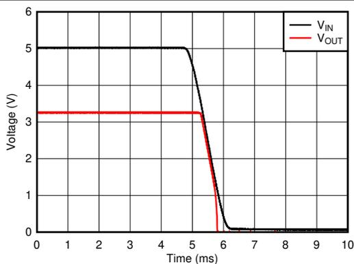
**Figure 5-11.  $V_{IN} = V_{EN}$  Shutdown**
