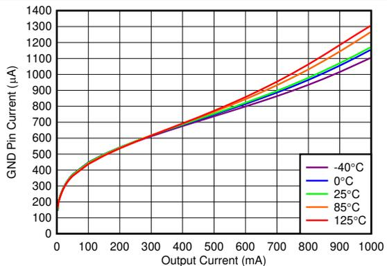
**Figure 5-18.  $I_{GND}$  vs  $I_{OUT}$**
