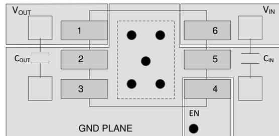
**Figure 7-8. Layout Example: DRV Package**
