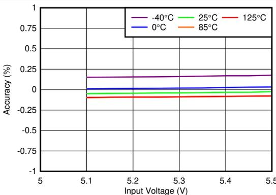
**Figure 5-17. 5.0V Accuracy vs  $V_{IN}$  (Line Regulation)**
