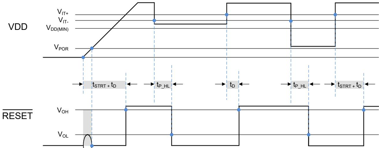
(1)  $t_{D (no\ cap)}$  is included in  $t_{STRT}$  time delay. If  $t_D$  delay is programmed by an external capacitor connected to CT pin then  $t_D$  programmed time will be added to the startup time,  $V_{DD}$  slew rate = 100 mV /  $\mu$ s.
