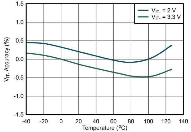
Figure 7-5. V<sub>IT-</sub> Accuracy vs Temperature
