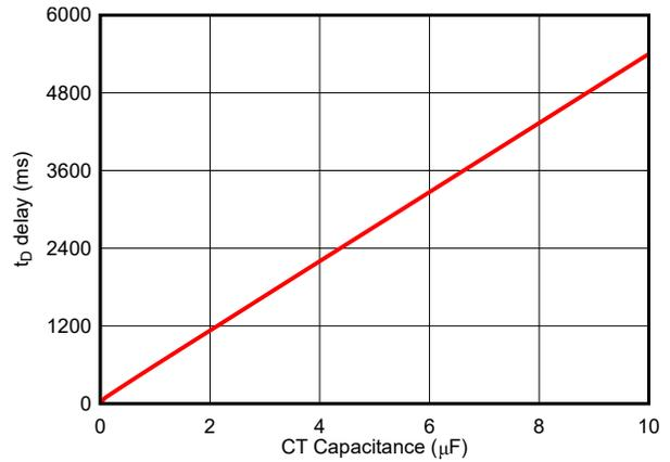
Figure 7-9. Reset Time Delay vs CT Capacitance
