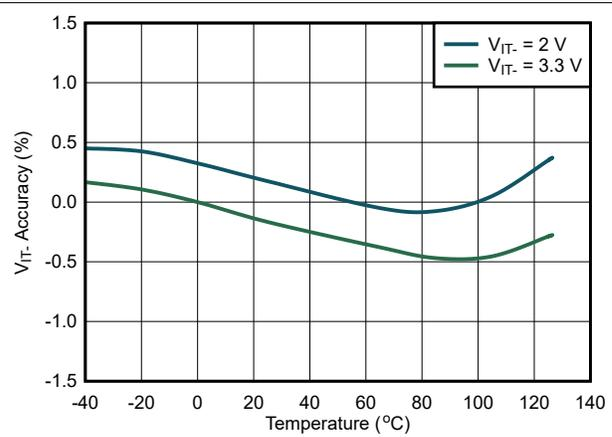
Figure 7-5. V<sub>IT-</sub> Accuracy vs Temperature
