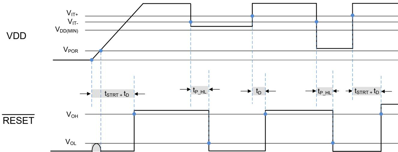
(4)  $t_{D (no\ cap)}$  is included in  $t_{STRT}$  time delay. If  $t_D$  delay is programmed by an external capacitor connected to CT pin then  $t_D$  programmed time will be added to the startup time,  $V_{DD}$  slew rate = 100 mV /  $\mu$ s.
