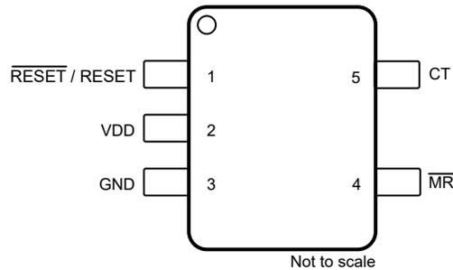
**Figure 6-1. Pin Configuration TLV840M-Q1
