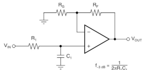
$$\frac{V_{\text{OUT}}}{V_{\text{IN}}} = \left(1 + \frac{R_{\text{F}}}{R_{\text{G}}}\right) \left(\frac{1}{1 + sR_1C_1}\right)$$
