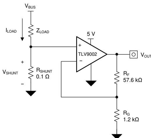
Figure 9-1. TLV900x in a Low-Side, Current-Sensing Application
