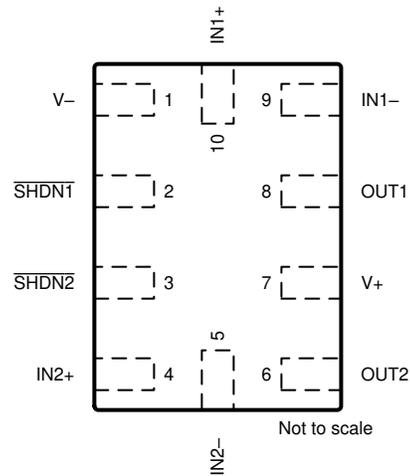
**Figure 6-9. TLV9002S RUG Package 10-Pin X2QFN Top View**
