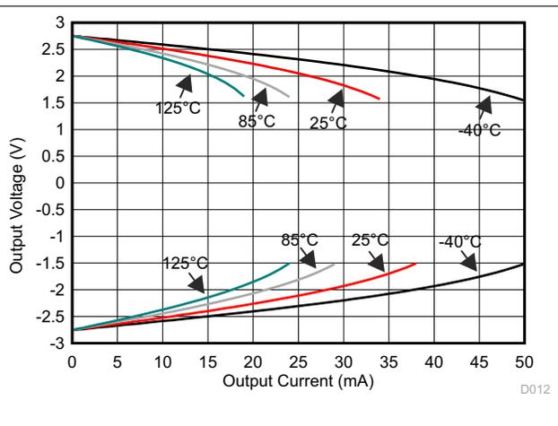
**Figure 7-12. Output Voltage vs Output Current (Claw)**
