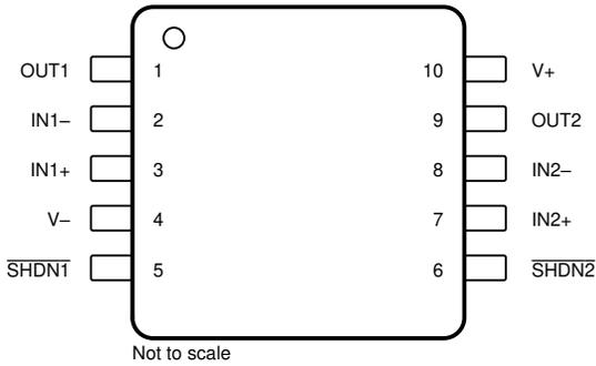
**Figure 6-8. TLV9002S DGS Package 10-Pin VSSOP Top View**
