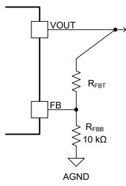
Figure 7-2. FB Resistor Divider
