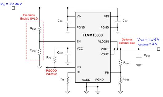
Figure 7-1. TLVM13630 Schematic Diagram with Input Voltage Operating Range of 3 V to 36 V
