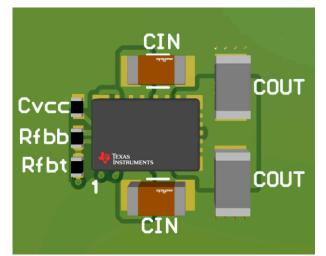
Figure 10-1. Typical Top-Layer Layout
