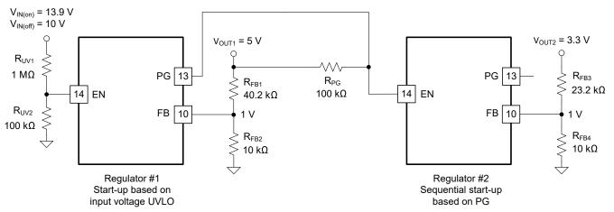
Figure 7-4. TLVM13630 Sequencing Implementation Using PG and EN
