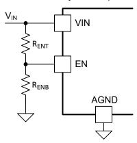
Figure 7-3. VIN UVLO Using the EN Pin
