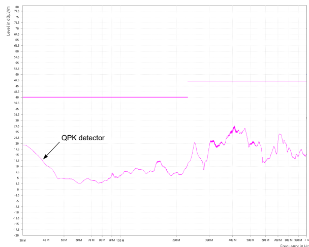
Figure 9-11. CISPR 32 Class B Radiated Emissions: Vertical Polarization
