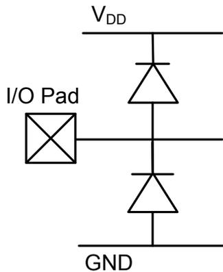
**Table 20-28. Non-Fail-Safe I/O Pad Voltage/Current Characteristics<sup>abcd</sup>**
