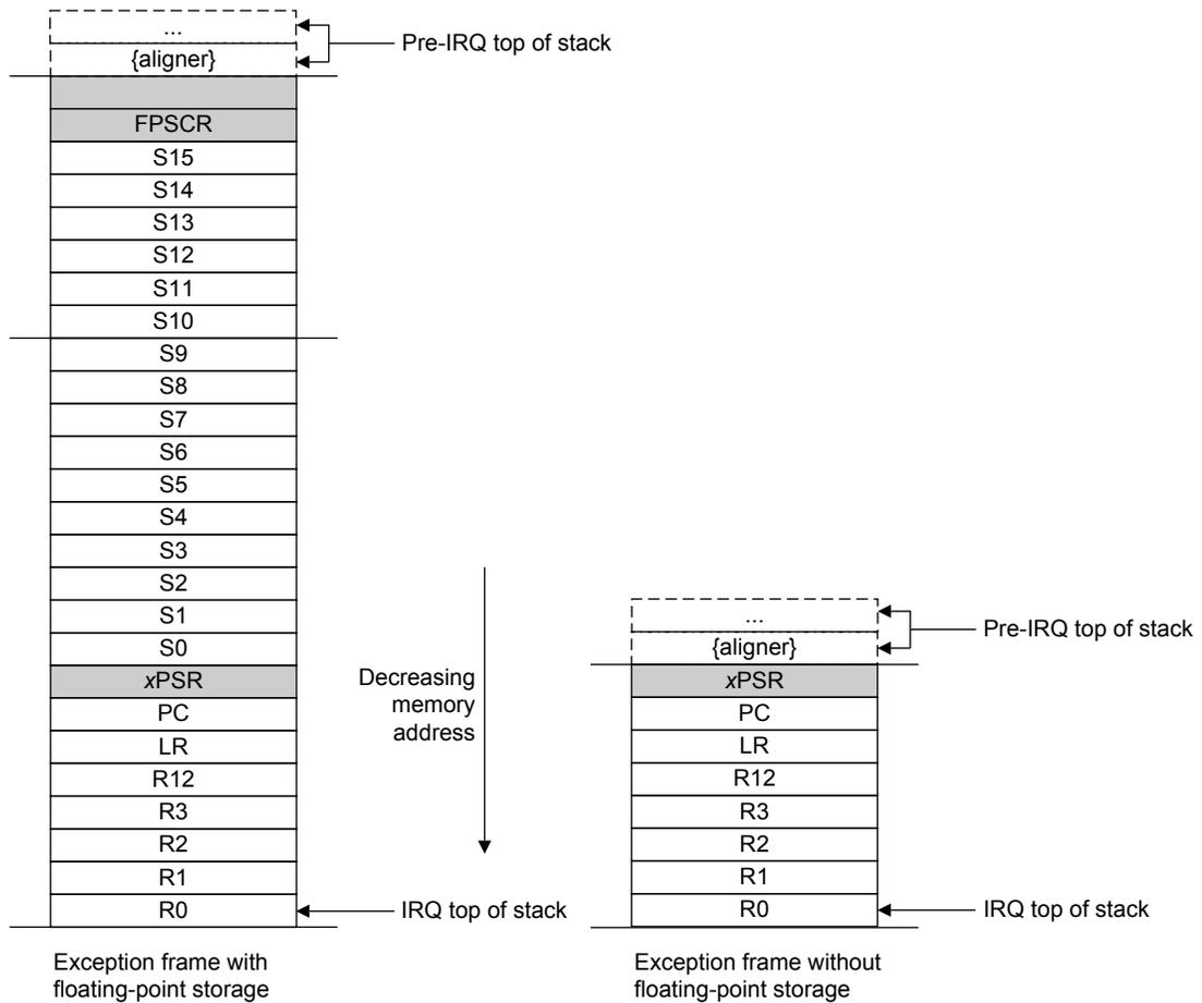
Immediately after stacking, the stack pointer indicates the lowest address in the stack frame.
