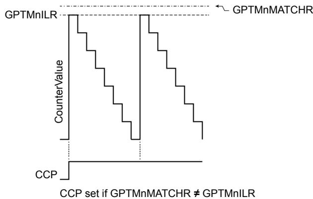
Figure 10-7 on page 639 shows how the CCP output operates when the **PLO** and **MRSU** bits are set and the **GPTMTnMATCHR** value is the same as the **GPTMTnILR** value. In this situation, if the **PLO** bit is 0, the CCP signal goes high when the **GPTMTnILR** value is loaded and the match would be essentially ignored.
