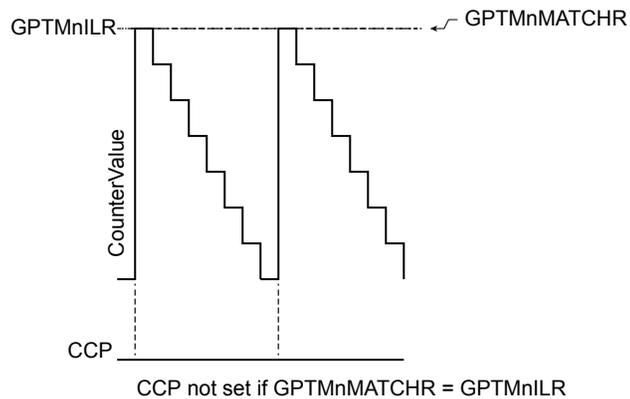
Figure 10-8 on page 639 shows how the CCP output operates when the `PLO` and `MRSU` bits are set and the **GPTMTnILR** is greater than the **GPTMTnMATCHR** value.
