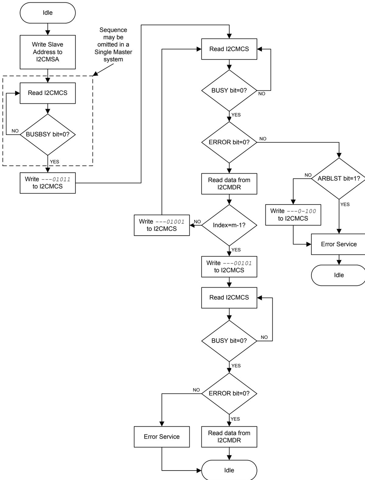
Figure 15-12. Master RECEIVE with Repeated START after Master TRANSMIT
