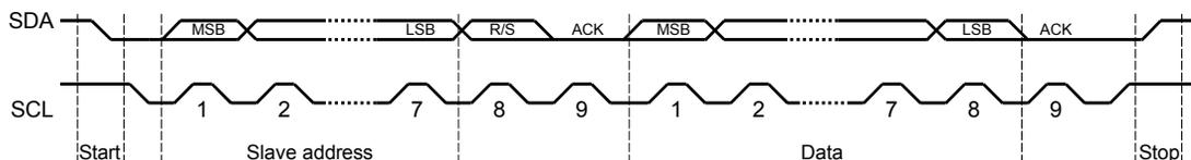
The first seven bits of the first byte make up the slave address (see Figure 15-5). The eighth bit determines the direction of the message. A zero in the R/S position of the first byte means that the
