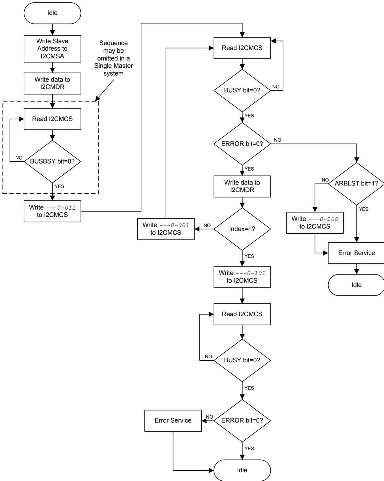
Figure 15-11. Master RECEIVE of Multiple Data Bytes
