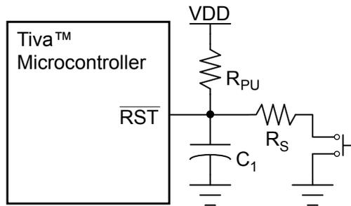
Typical  $R_{PU} = 10\text{ k}\Omega$
