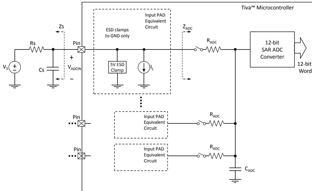
The ADC operates from both the 3.3-V analog and 1.2-V digital power supplies. The ADC clock can be configured to reduce power consumption when ADC conversions are not required (see “System Control” on page 211). The analog inputs are connected to the ADC through specially balanced input paths to minimize the distortion and cross-talk on the inputs. Detailed information on the ADC power supplies and analog inputs can be found in “Analog-to-Digital Converter (ADC)” on page 1084.
