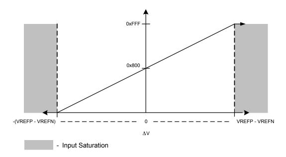
Figure 13-10. Differential Voltage Representation
