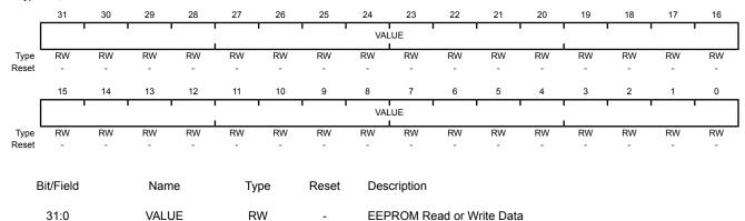
On a read, this field contains the value at the word pointed to by **EEOFFSET**. On a write, this field contains the data to be stored at the word pointed to by **EEOFFSET**. For writes, configuring this field starts the write process. If protection and access rules do not permit reads, all 1s are returned. If protection and access rules do not permit writes, the write fails and the **EEDONE** register indicates failure.
