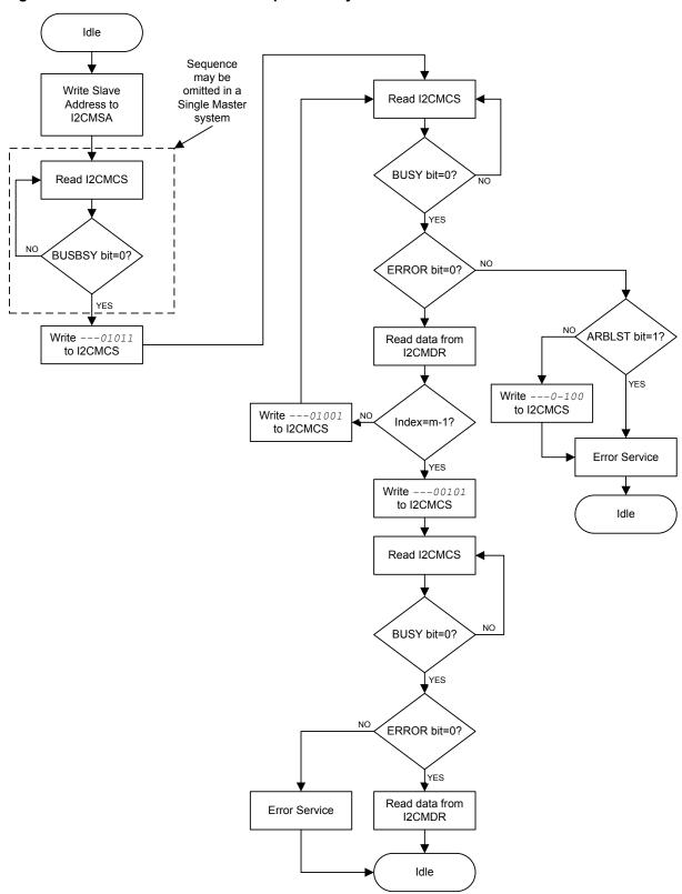
Figure 16-11. Master RECEIVE of Multiple Data Bytes
