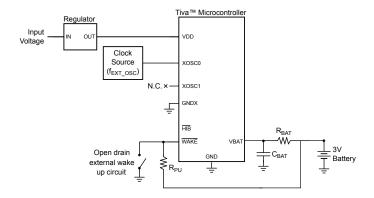
Note: Some devices may not supply the GNDX, WAKE or HIB signals. See "Signal Tables" on page 1076 for pins specific to your device.
