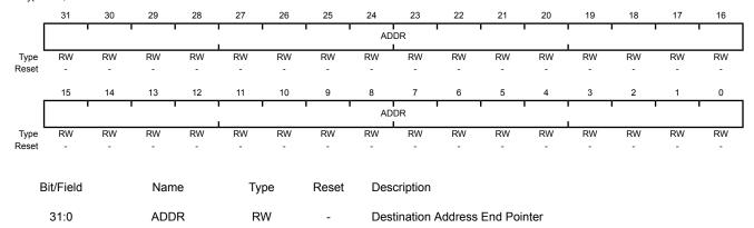
This field points to the last address of the  $\mu DMA$  transfer destination (inclusive). If the destination address is not incrementing (the <code>DSTINC</code> field in the **DMACHCTL** register is 0x3), then this field points at the destination location itself (such as a peripheral data register).
