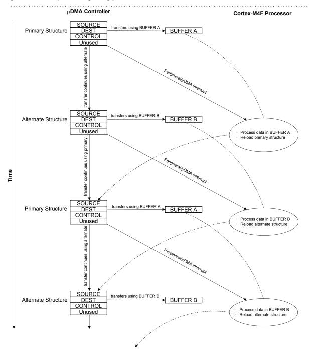
Figure 9-2. Example of Ping-Pong µDMA Transaction
