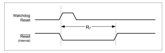
Figure 21-14. MOSC Failure Reset Timing
