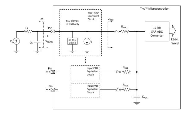
The ADC operates from both the 3.3-V analog and 1.2-V digital power supplies. The ADC clock can be configured to reduce power consumption when ADC conversions are not required (see "System Control" on page 215). The analog inputs are connected to the ADC through specially balanced input paths to minimize the distortion and cross-talk on the inputs. Detailed information on the ADC power supplies and analog inputs can be found in "Analog-to-Digital Converter (ADC)" on page 1127.
