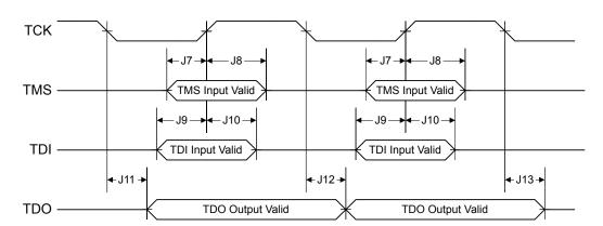
Figure 21-3. JTAG Test Access Port (TAP) Timing
