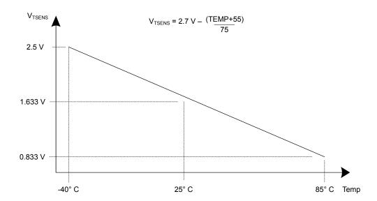
Figure 13-11. Internal Temperature Sensor Characteristic
