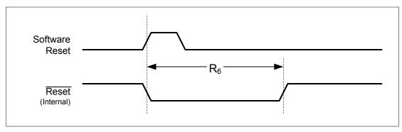
Figure 21-13. Watchdog Reset Timing
