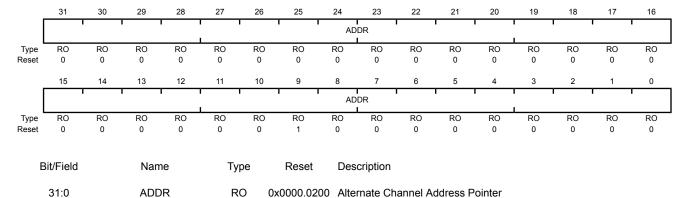
This field provides the base address of the alternate channel control structures.
