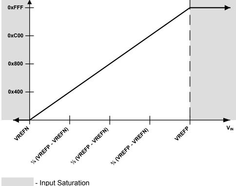
Figure 13-9. ADC Conversion Result
