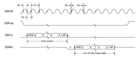
Figure 21-21. Master Mode SSI Timing for SPI Frame Format (FRF=00), with SPH=1
