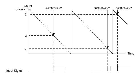
Figure 11-4. 16-Bit Input Edge-Time Mode Example
