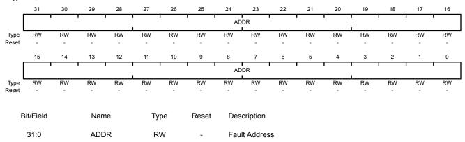
When the FAULTADDRV bit of **BFAULTSTAT** is set, this field holds the address of the location that generated the bus fault.
