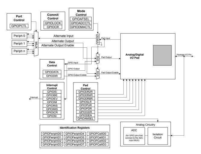
Figure 10-2. Analog/Digital I/O Pads
