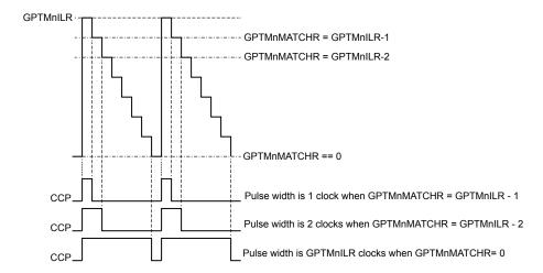
Figure 11-8. CCP Output, GPTMTnILR > GPTMTnMATCHR
