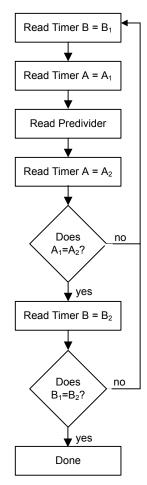
Figure 11-2. Reading the RTC Value
