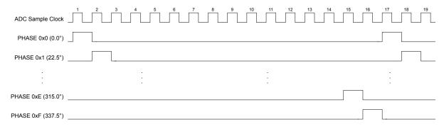
This feature can be used to double the sampling rate of an input. Both ADC module 0 and ADC module 1 can be programmed to sample the same input. ADC module 0 could sample at the standard position (the PHASE field in the **ADCSPC** register is 0x0). ADC module 1 can be configured to sample at 180 (PHASE = 0x8). The two modules can be be synchronized using the GSYNC and SYNCWAIT
