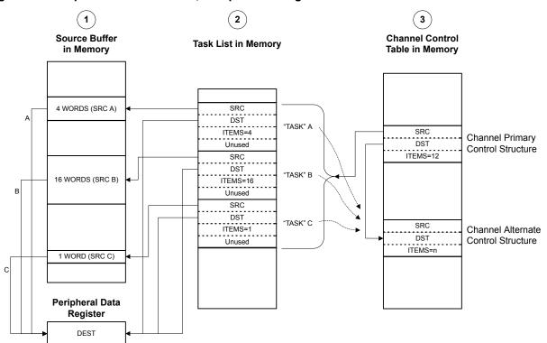
Figure 9-5. Peripheral Scatter-Gather, Setup and Configuration
