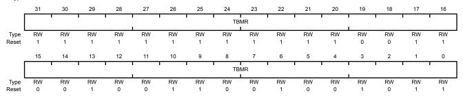
Bit/Field Name Type Reset Description 31:0 **TBMR** 0x0000.FFFF GPTM Timer B Match Register RW
