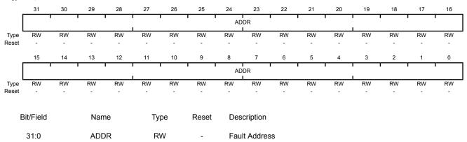
When the MMARV bit of **MFAULTSTAT** is set, this field holds the address of the location that generated the memory management fault.
