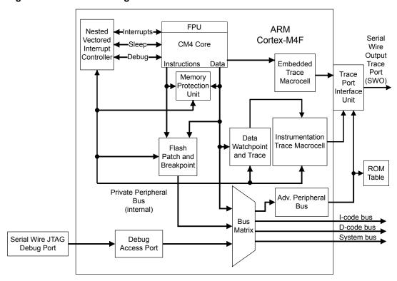
Figure 2-1. CPU Block Diagram
