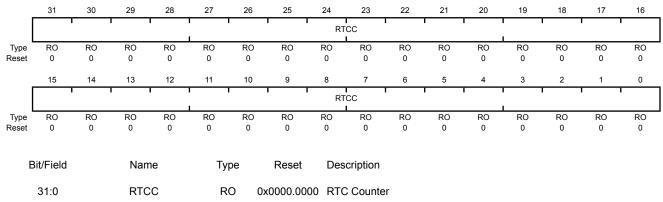
A read returns the 32-bit counter value, which represents the seconds elapsed since the RTC was enabled. This register is read-only. To change the value, use the **HIBRTCLD** register.
