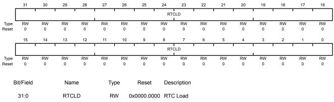
A write loads the current value into the RTC counter (RTCC).
