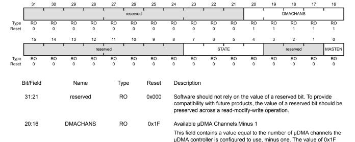
15:8 RO 0x00 Software should not rely on the value of a reserved bit. To provide reserved compatibility with future products, the value of a reserved bit should be preserved across a read-modify-write operation.
