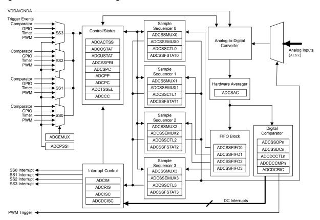
Figure 13-2. ADC Module Block Diagram
