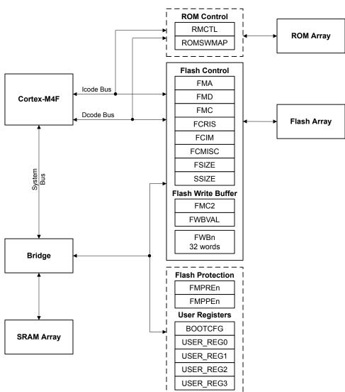
Figure 8-1. Internal Memory Block Diagram
