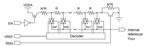
**Note:** In the figure above, N\*R represents a multiple of the R value that produces the results specified in Table 18-2 on page 1063.
