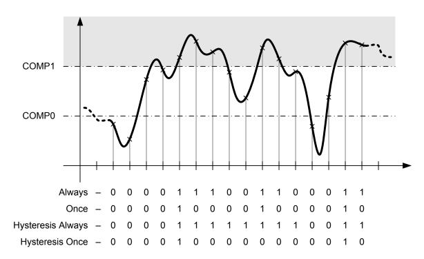
Figure 13-14. High-Band Operation (CIC=0x3)
