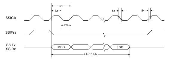
Figure 21-20. SSI Timing for MICROWIRE Frame Format (FRF=10), Single Transfer
