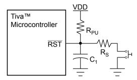
Typical  $R_{PU} = 10 \text{ k}\Omega$
