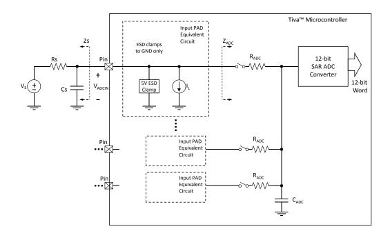
Figure 21-18. ADC Input Equivalency Diagram
