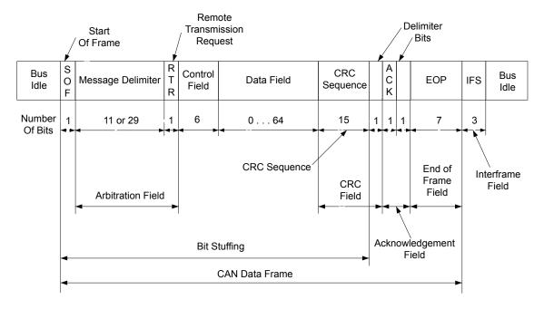
The protocol controller transfers and receives the serial data from the CAN bus and passes the data on to the message handler. The message handler then loads this information into the appropriate message object based on the current filtering and identifiers in the message object memory. The message handler is also responsible for generating interrupts based on events on the CAN bus.
