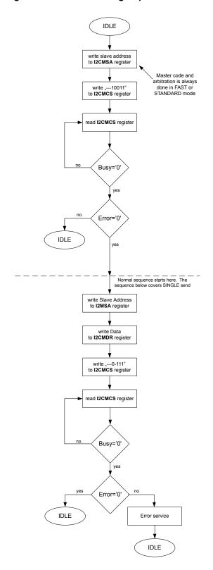
Figure 16-14. Standard High Speed Mode Master Transmit
