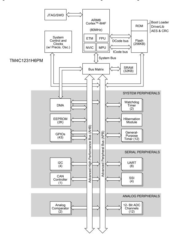
Figure 1-1. Tiva<sup>™</sup> TM4C1231H6PM Microcontroller High-Level Block Diagram
