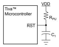
$R_{PU}$  = 1 k $\Omega$  to 100 k $\Omega$
