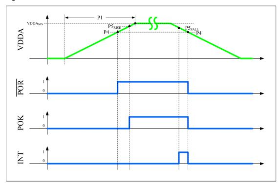
Figure 21-4. Power Assertions versus VDDA Levels
