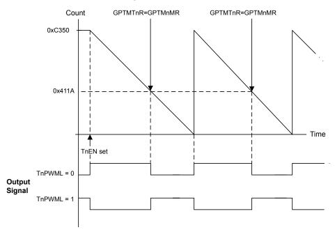
Figure 11-5. 16-Bit PWM Mode Example
