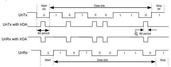
Figure 14-3. IrDA Data Modulation
