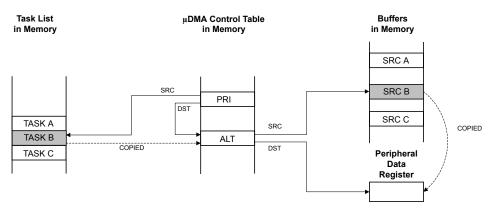
Using the channel's primary control structure, the  $\mu DMA$  controller copies task B configuration to the channel's alternate control structure.
