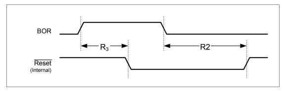
Figure 21-11. External Reset Timing (RST)
