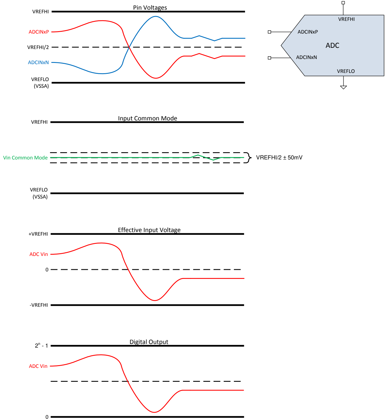
Figure 6-35. Differential Signaling Mode
