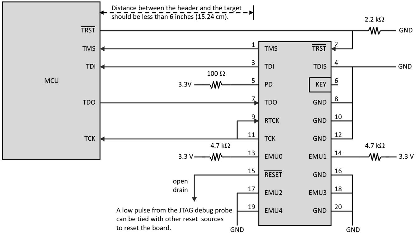
**Figure 6-14. Connecting to the 20-Pin JTAG Header**
