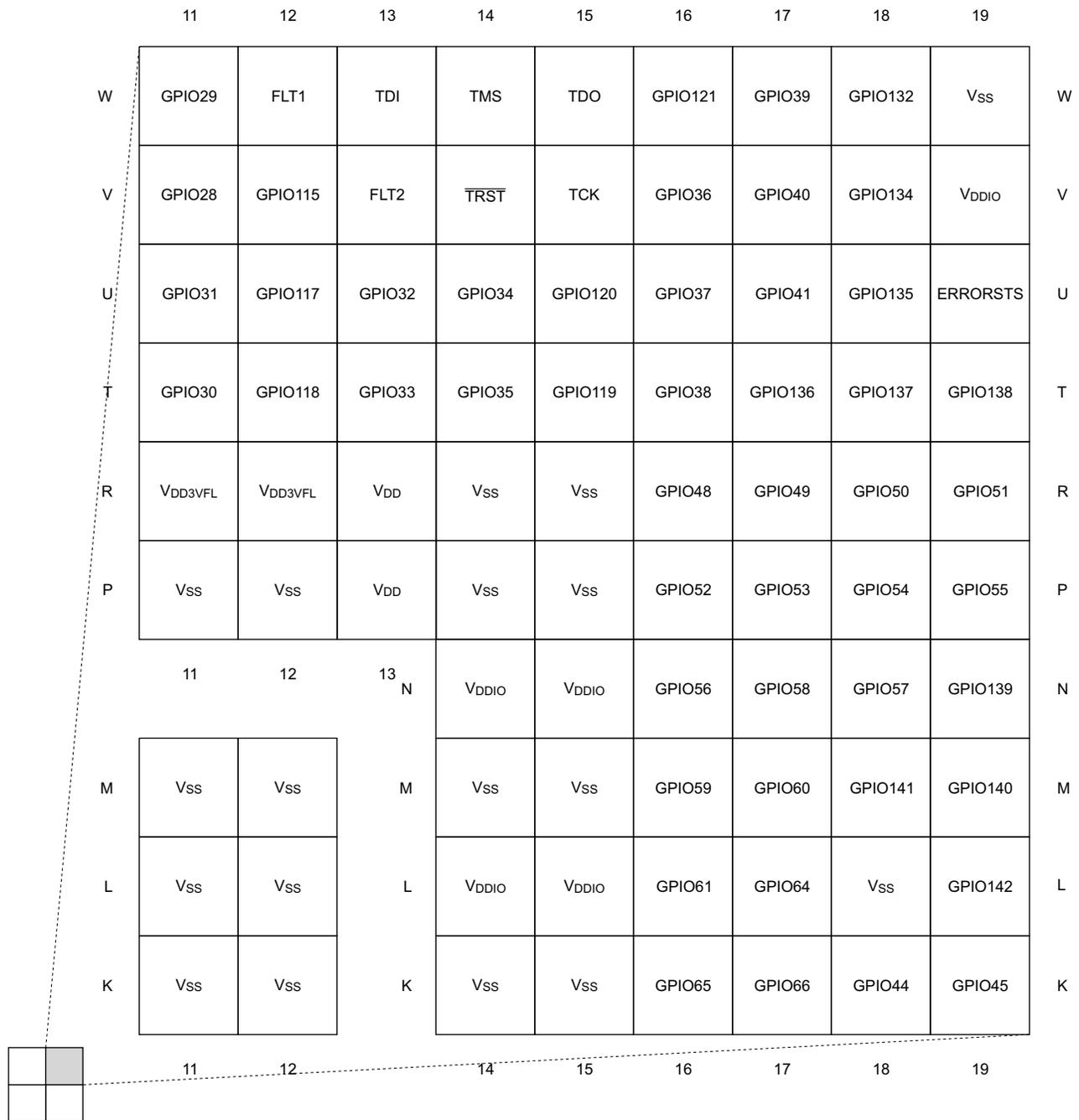
A. Only the GPIO function is shown on GPIO terminals. See [Section 5.2.1](#) for the complete, muxed signal name.
