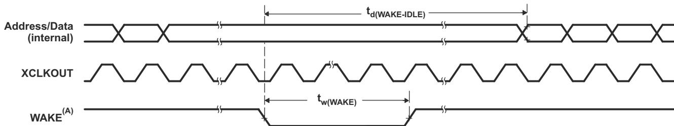
A. WAKE can be any enabled interrupt,  $\overline{WDINT}$  or  $\overline{XRS}$ . After the IDLE instruction is executed, a delay of five OSCCLK cycles (minimum) is needed before the wake-up signal could be asserted.
