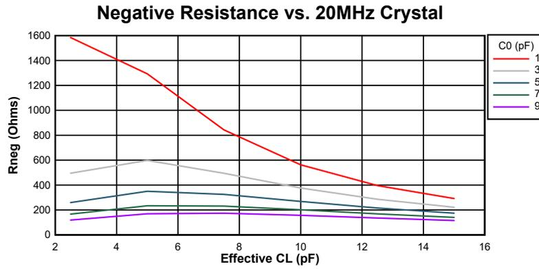
**Figure 6-12. Negative Resistance Variation at 20 MHz**
