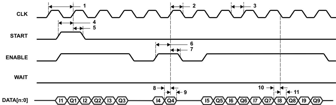
Figure 6-85. uPP Double Data Rate (DDR) Receive Timing
