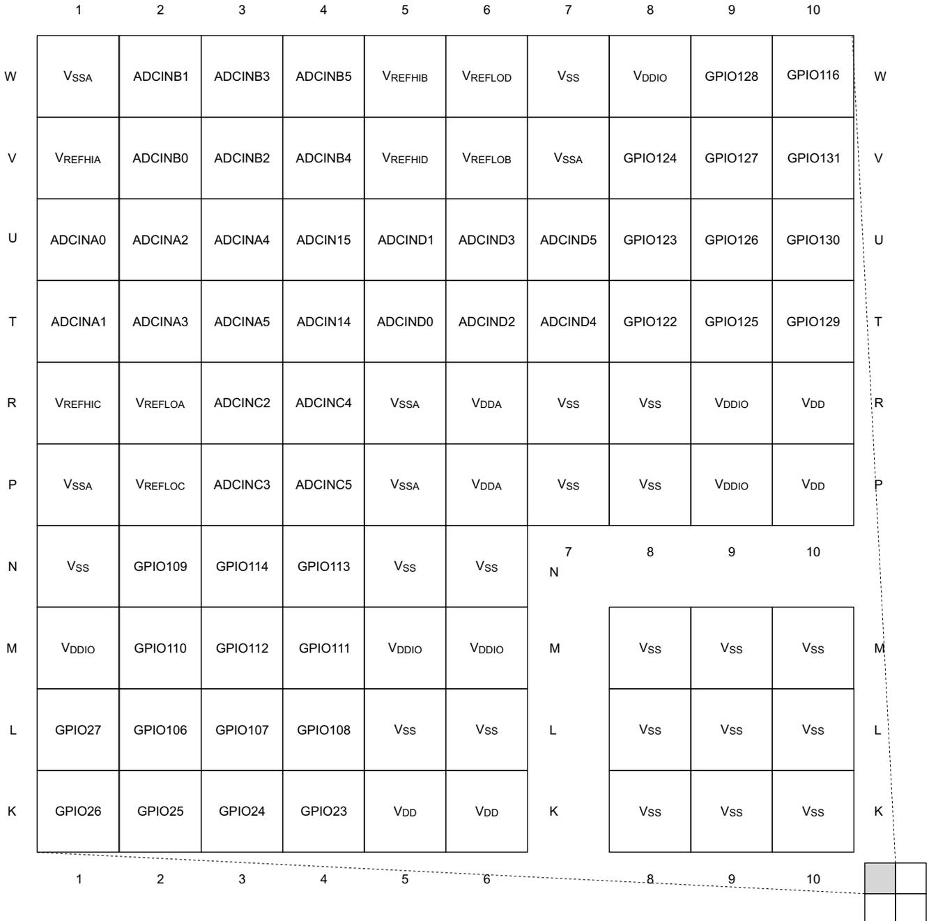
A. Only the GPIO function is shown on GPIO terminals. See Section 5.2.1 for the complete, muxed signal name.
