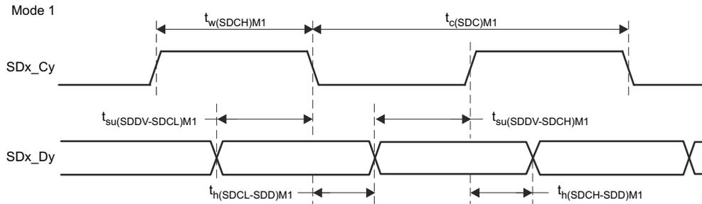
**Figure 6-62. SDFM Timing Diagram – Mode 1**
