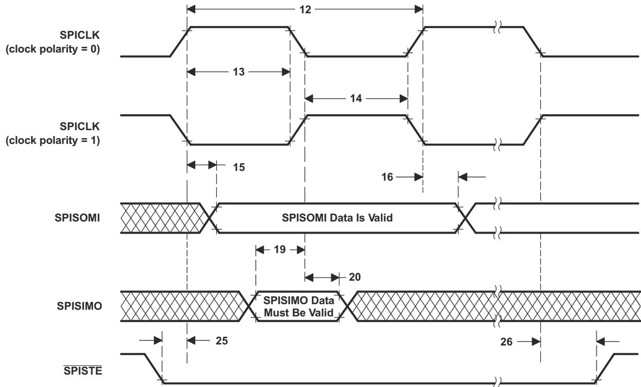
**Figure 6-79. SPI Slave Mode External Timing (Clock Phase = 0)**
