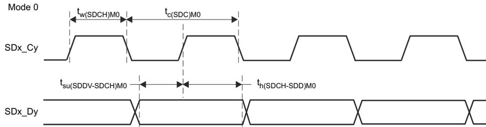
**Figure 6-61. SDFM Timing Diagram – Mode 0**
