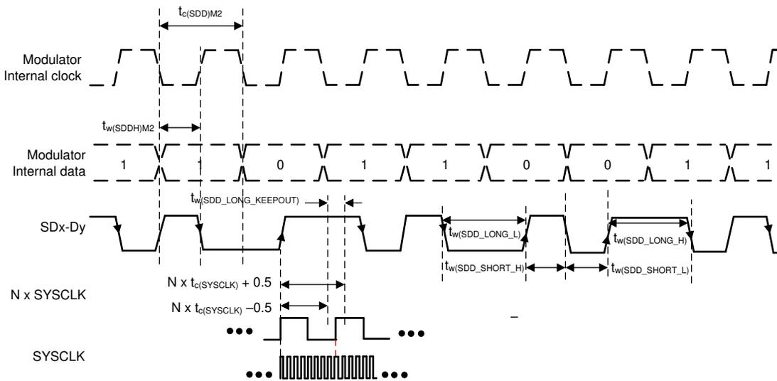
**Figure 6-63. SDFM Timing Diagram – Mode 2**
