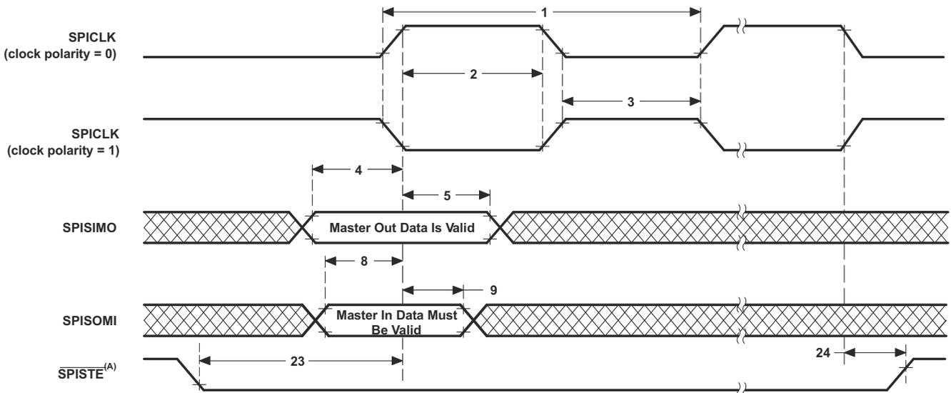
A. On the trailing end of the word,  $\overline{\text{SPISTE}}$  will go inactive except between back-to-back transmit words in both FIFO and non-FIFO modes.
