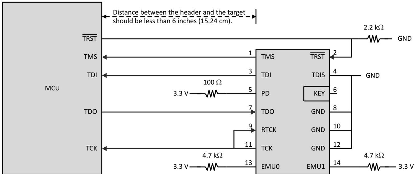
**Figure 6-13. Connecting to the 14-Pin JTAG Header**
