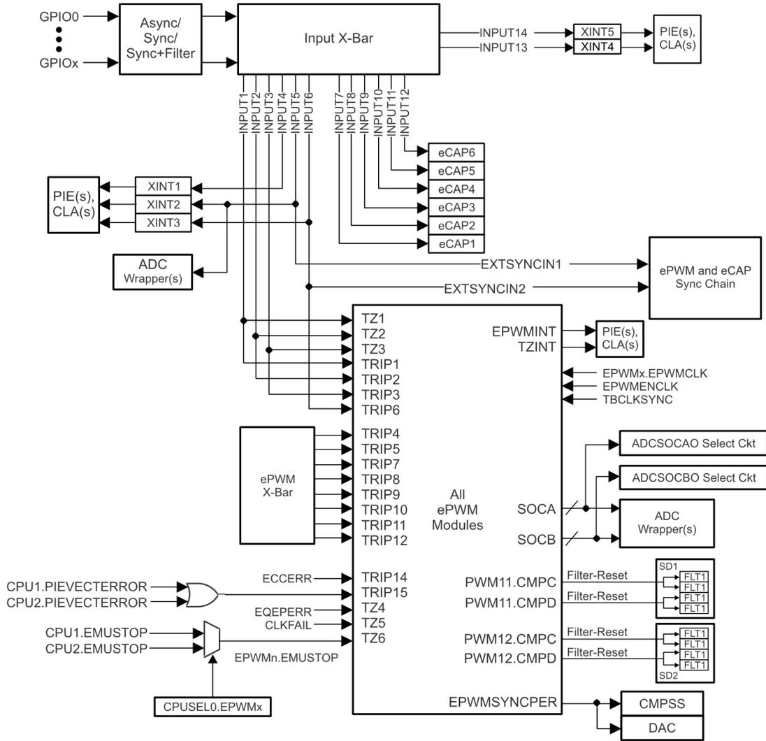
**Figure 6-55. ePWM Trip Input Connectivity**
