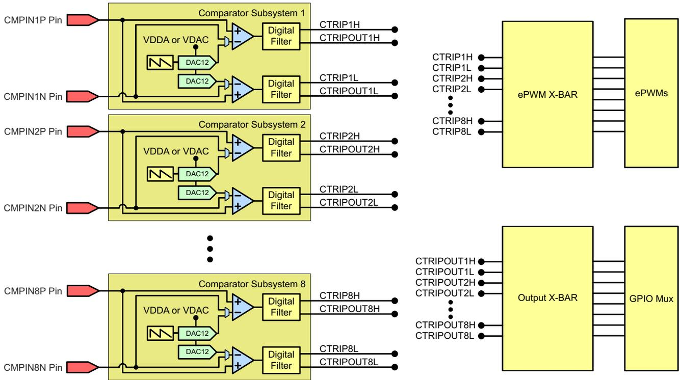
**Figure 6-41. CMPSS Connectivity (337-Ball ZWT and 176-Pin PTP)**
