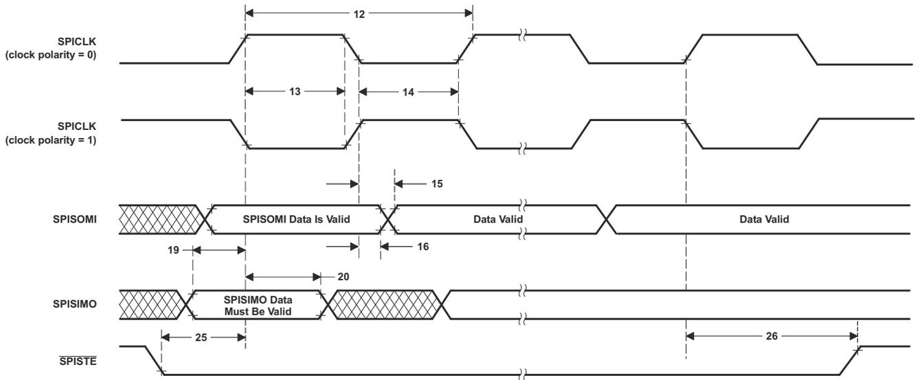
**Figure 6-80. SPI Slave Mode External Timing (Clock Phase = 1)**
