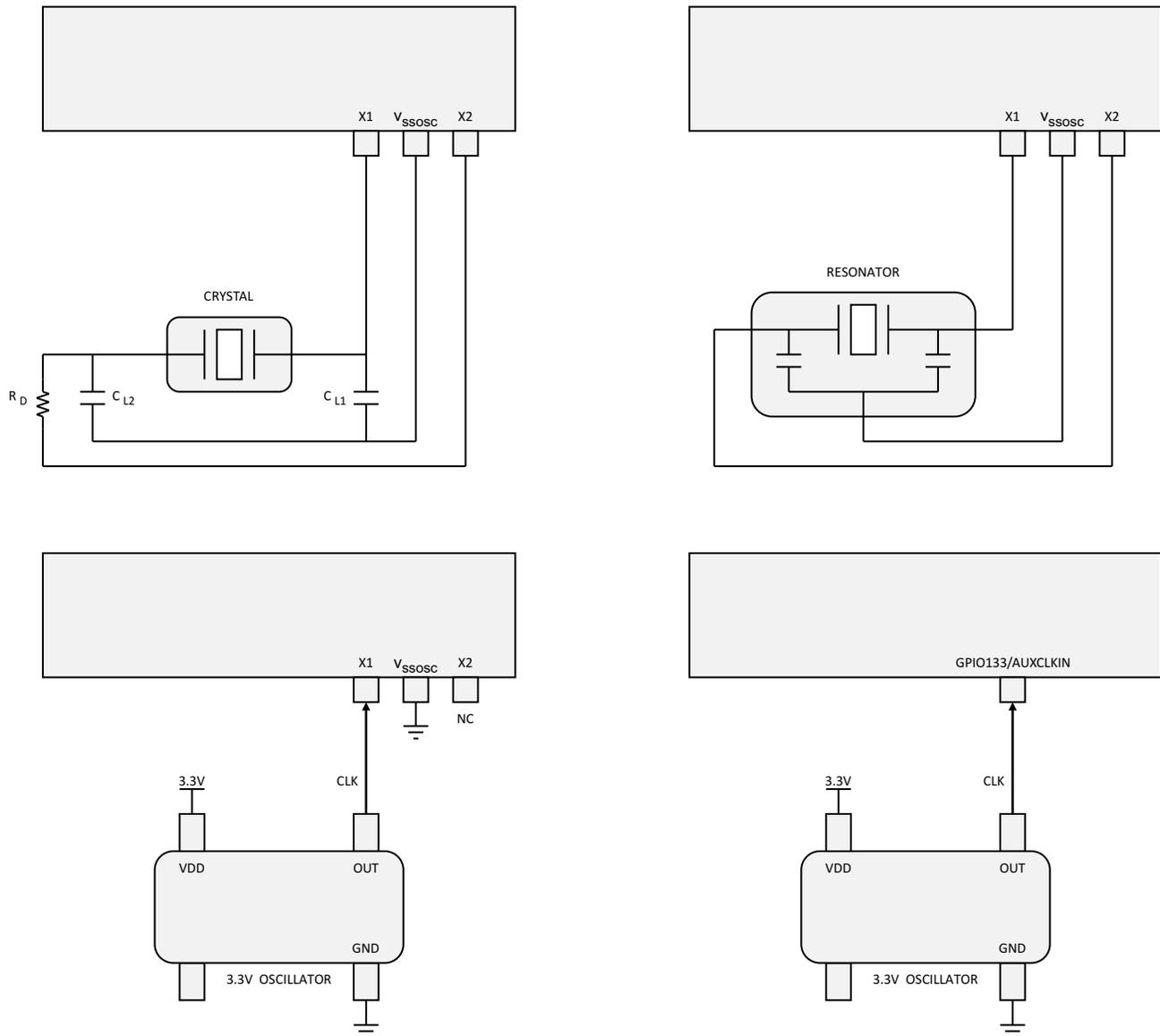
**Figure 6-8. Connecting Input Clocks to a 2837xD Device**
