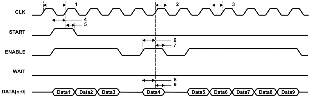
Figure 6-84. uPP Single Data Rate (SDR) Receive Timing
