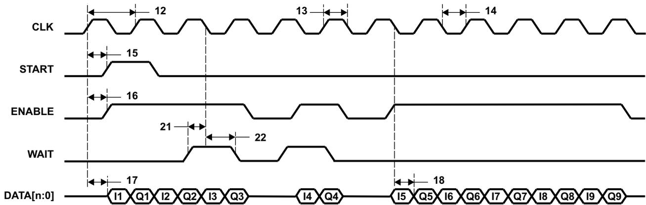
Figure 6-87. uPP Double Data Rate (DDR) Transmit Timing
