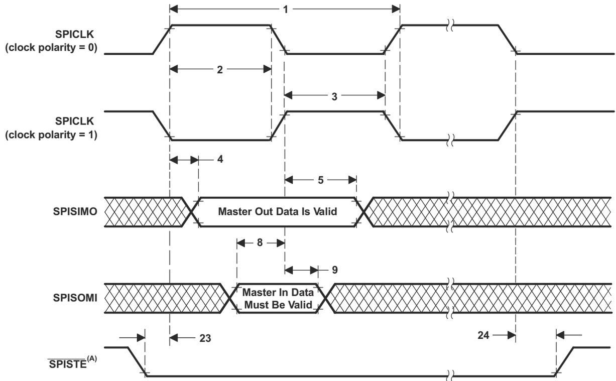
A. On the trailing end of the word,  $\overline{\text{SPISTE}}$  will go inactive except between back-to-back transmit words in both FIFO and non-FIFO modes.
