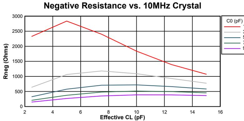
**Figure 6-11. Negative Resistance Variation at 10 MHz**
