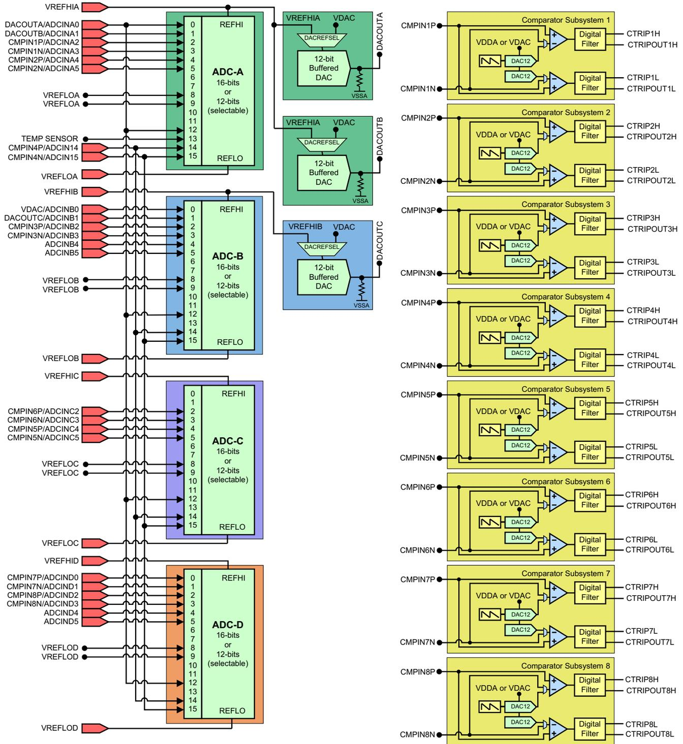
Figure 6-31. Analog Subsystem Block Diagram (337-Ball ZWT)
