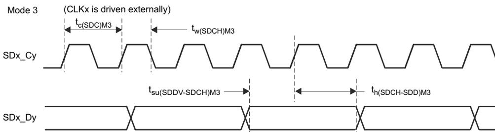
**Figure 6-64. SDFM Timing Diagram – Mode 3**
