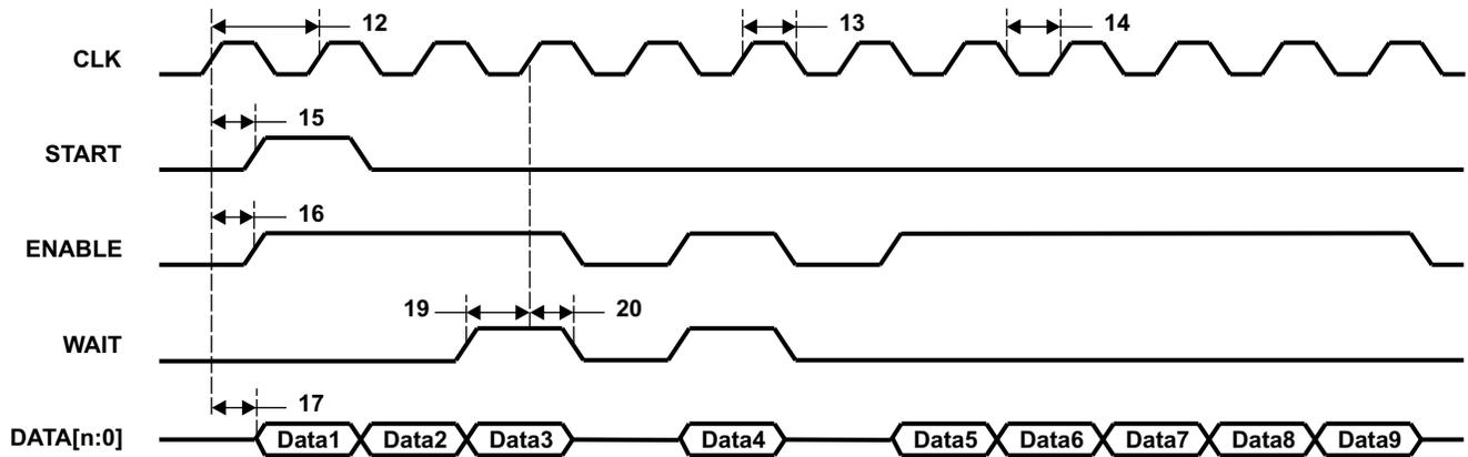
Figure 6-86. uPP Single Data Rate (SDR) Transmit Timing
