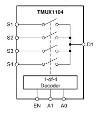
Figure 7-1. TMUX1104 Functional Block Diagram
