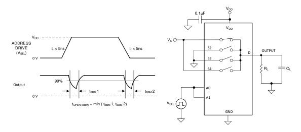
Figure 6-5. Break-Before-Make Delay Measurement Setup
