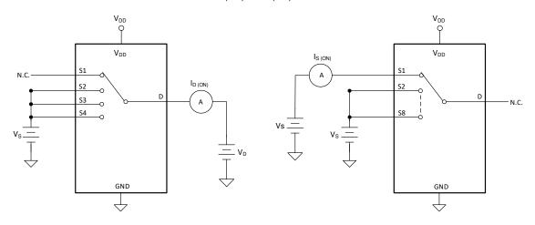
Figure 6-3. On-Leakage Measurement Setup
