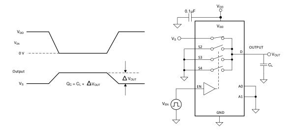
Figure 6-7. Charge-Injection Measurement Setup
