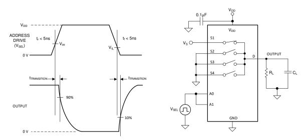
Figure 6-4. Transition-Time Measurement Setup
