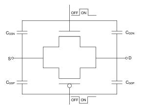
Figure 7-3. Transmission Gate Topology
