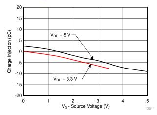
Figure 7-4. Charge Injection vs Source Voltage
