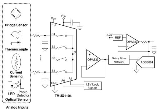
Figure 8-1. Multiplexing Signals to External ADC
