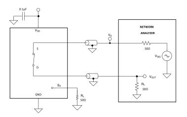
Figure 6-10. Bandwidth Measurement Setup
