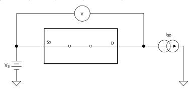
Figure 6-1. On-Resistance Measurement Setup
