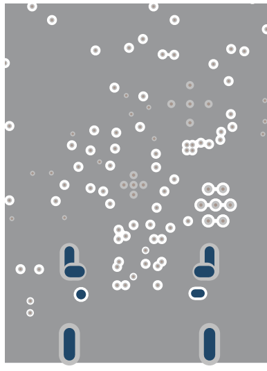
Figure 7-6. TPS26750 PCB Layout - GND Layer 2
