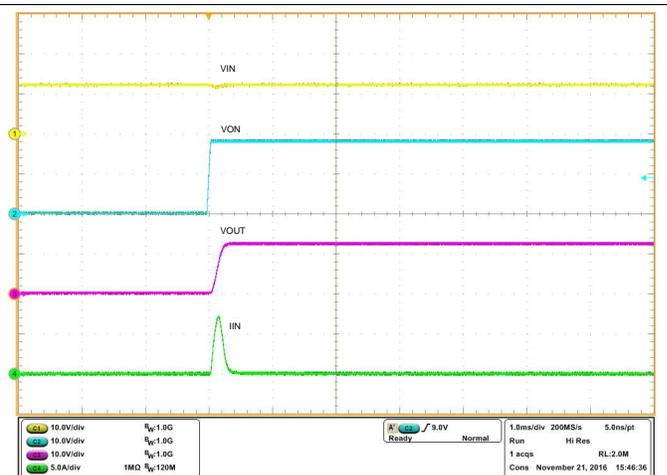
Figure 31. TPS22810 Inrush Current With  $C_L = 100\ \mu\text{F}$ ,  $CT = 0\ \text{pF}$
