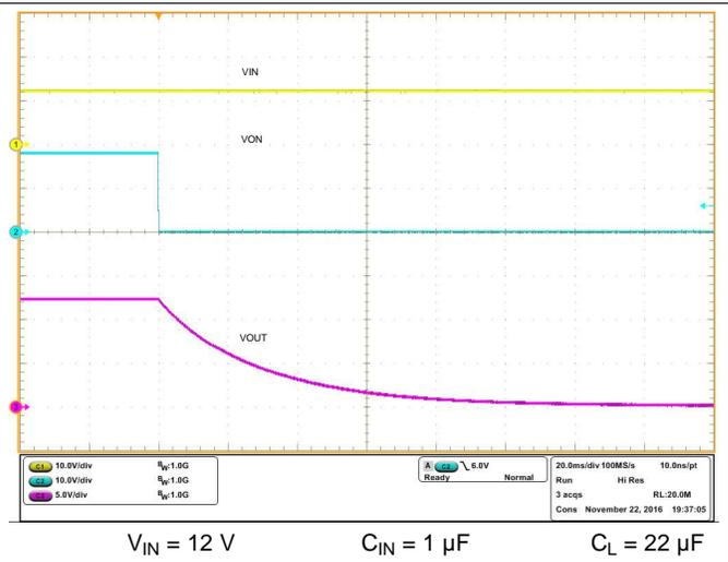
Figure 25.  $t_F$  at  $V_{IN} = 12\text{ V}$ ,  $R_{QOD} = 1000\ \Omega$
