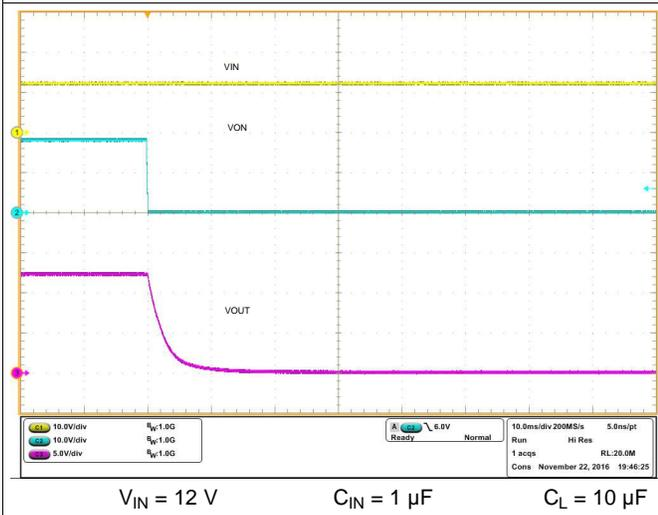
Figure 24.  $t_F$  at  $V_{IN} = 12\text{ V}$ ,  $QOD = V_{OUT}$
