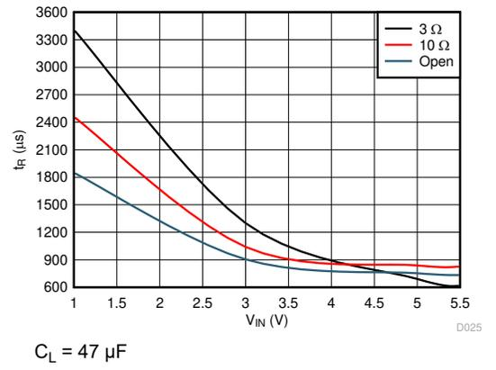
Figure 7-22. Rise Time vs Load Resistance (CT = 10000 pF)
