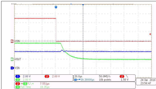
Figure 7-25. Turn-Off at 3.6 V
