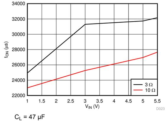
Figure 7-20. Turn-On vs Load Resistance (CT = 10000 pF)
