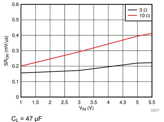
Figure 7-24. Slew Rate vs Load Resistance (CT = 10000 pF)
