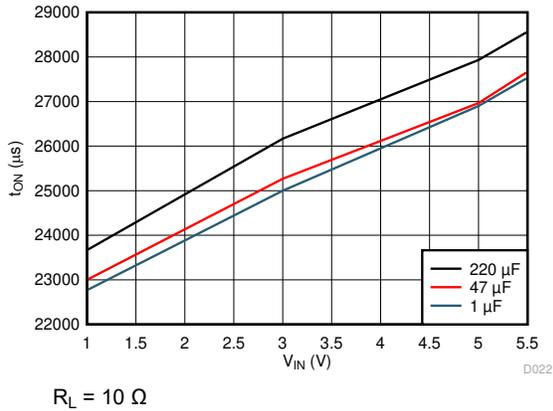
Figure 7-19. Turn-On vs Load Capacitance (CT = 10000 pF)
