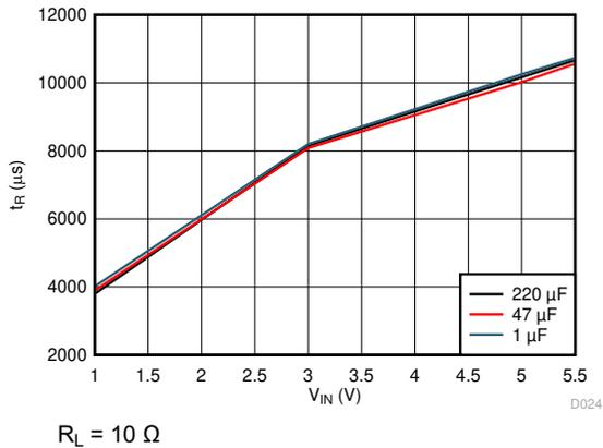
Figure 7-21. Rise Time vs Load Capacitance (CT = 10000 pF)
