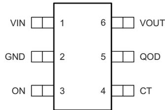
Figure 6-1. DBV Package 6-Pin SOT-23 Top View
