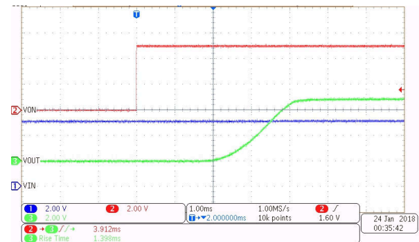
Figure 7-14. Turn-On at 5 V (CT = 1000 pF)
