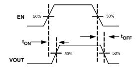
Figure 16. VOUT Enable Timing
