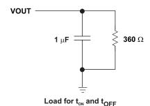
Figure 14. Test Circuit and  $t_{\text{ON}}$  /  $t_{\text{OFF}}$  Waveforms
