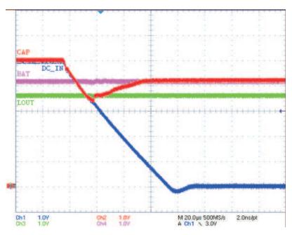
Figure 19. DC\_IN Removed, BAT Powers LDO (LOUT = 3.6 V)
