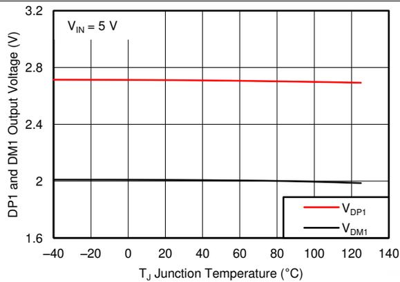
Figure 5. DP1 and DM1 Output Voltage vs Temperature
