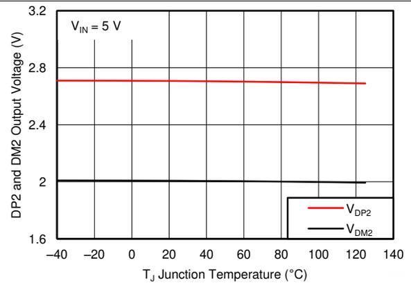
Figure 6. DP2 and DM2 Output Voltage vs Temperature
