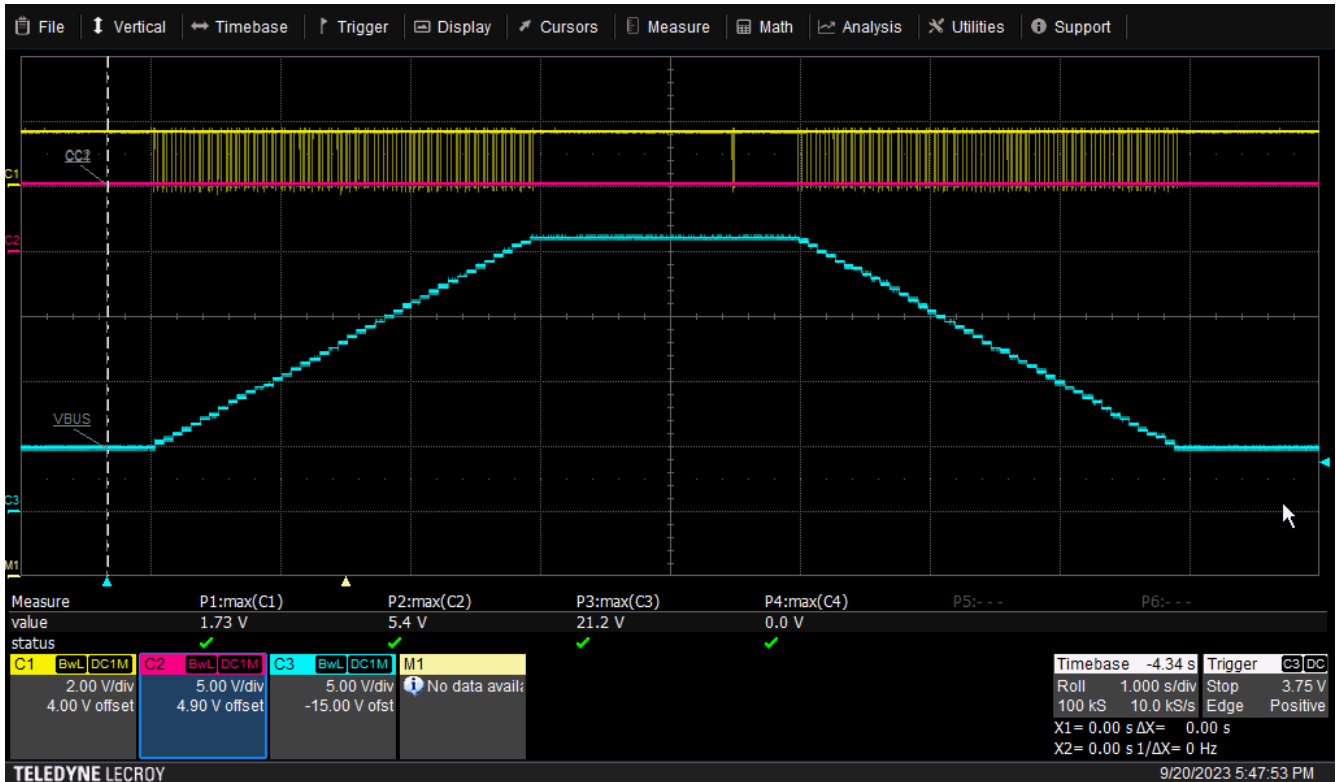
Figure 9-14. PPS PD Negotiation VBUS Increasing/Decreasing
