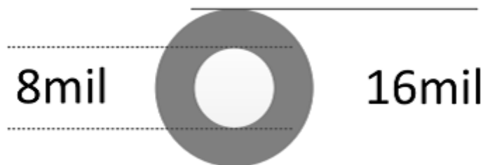
Figure 11-6. Recommended Minimum Via Sizing
