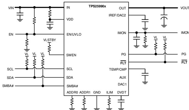
Figure 9-1. Single Device, Standalone Operation
