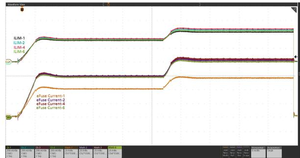
**Figure 9-12. Circuit-Breaker Response (Current distribution among six devices in parallel):**  $V_{IN} = 12\text{ V}$ ,  $t_{OC\_TIMER} = 17\text{ ms}$ ,  $C_{LOAD} = 50\text{ mF}$ ,  $R_{IMON} = 150\ \Omega$ ,  $V_{IREF} = 1\text{ V}$ , and Load Current Stepped from 333 A to 530 A for more than 17 ms
