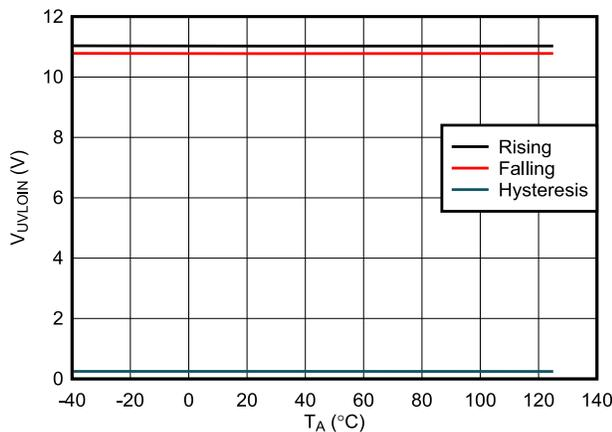
Figure 7-5. VIN Undervoltage Thresholds Across Temperature (VIN\_UV\_FLT = 0x8D)
