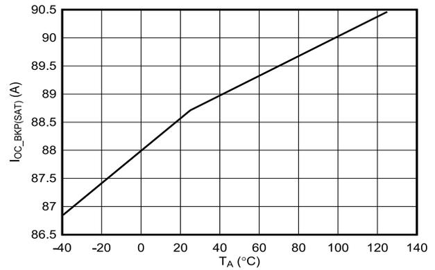
Figure 7-20. Backup Overcurrent Protection Threshold (Startup) Accuracy
