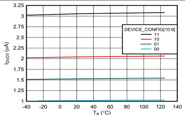
Figure 7-22. DVDT Pin Charging Current Across Temperature
