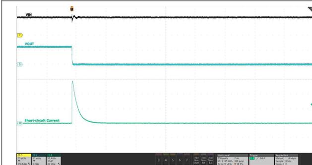
Device in steady-state, OUT shorted to GND. OCP threshold set to 55 A, Short-circuit fast recovery disabled (Default, DEVICE\_CONFIG[13] = 0b)
