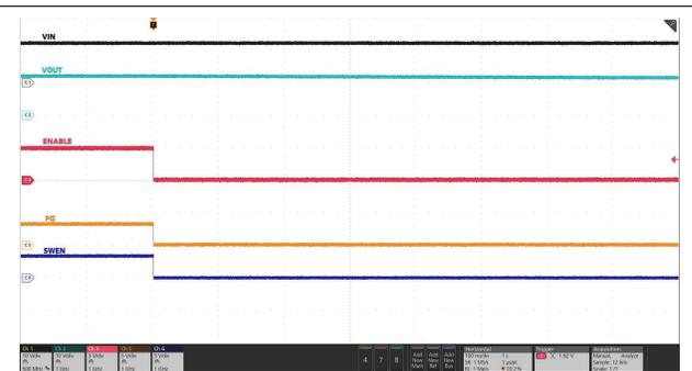
IN supply held steady at 12 V, EN pin toggled from high to low.
