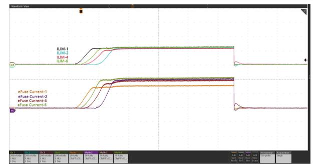
**Figure 9-8. Power Up into Short (Current distribution among six devices in parallel):  $V_{IN} = 12$  V, EN/UVLO Stepped Up From 0 V to 3 V,  $V_{IREF} = 1$  V,  $R_{ILIM(TPS25990)} = 422 \Omega$ ,  $R_{ILIM(TPS25985)} = 316 \Omega$ , and OUT Shorted to GND**
