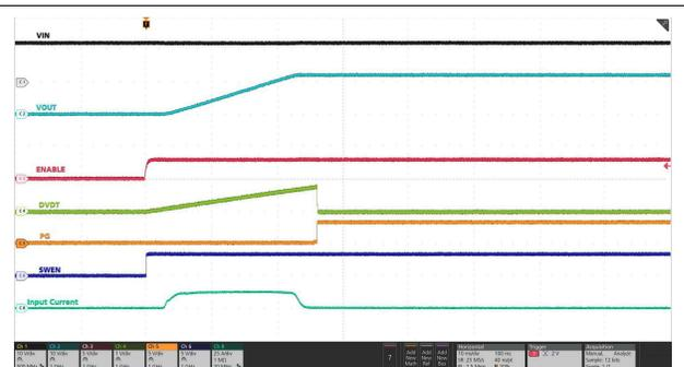
IN supply held steady at 12 V, EN toggled from low to high.  $C_{OUT} = 18\text{ mF}$ ,  $C_{dVdt} = 33\text{ nF}$ , DVDT scaling at 50 % ( $DEVICE\_CONFIG[10:9] = 00b$ )
