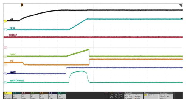
EN held high, IN supply ramped up to 12 V. C<sub>OUT</sub> = 18 mF, C<sub>dVdt</sub> = 33 nF
