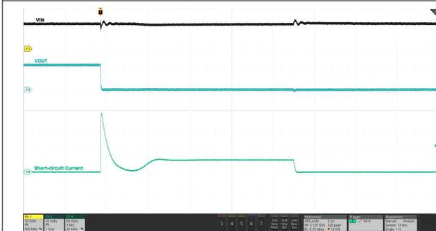
Device in steady-state, OUT shorted to GND. OCP threshold set to 55 A, Short-circuit fast recovery enabled (Default, DEVICE\_CONFIG[13] = 1b)
