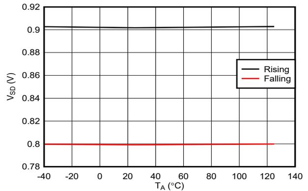
**Figure 7-10. EN/UVLO Based Shutdown Thresholds Across Temperature**
