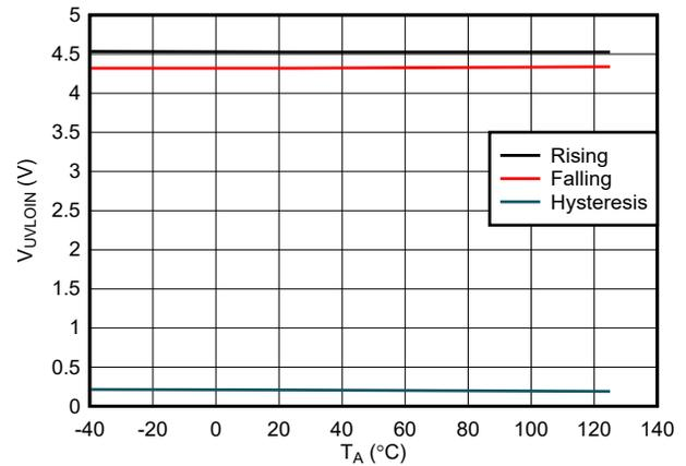
Figure 7-4. VIN Undervoltage Thresholds Across Temperature (VIN\_UV\_FLT = 0x38)
