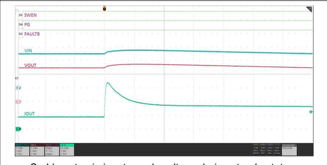
Sudden step in input supply voltage during steady-state causes output current spike without triggering a false fast-trip.
