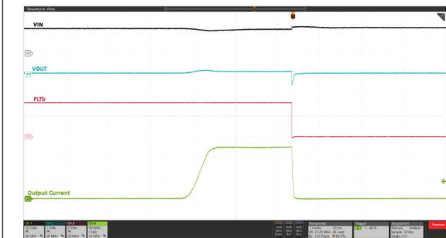
**Figure 9-7. Power Up into Short:  $V_{IN} = 12$  V, EN/UVLO Stepped Up From 0 V to 3 V,  $V_{IREF} = 1$  V,  $R_{ILIM(TPS25990)} = 422 \Omega$ ,  $R_{ILIM(TPS25985)} = 316 \Omega$ , and OUT Shorted to GND**
