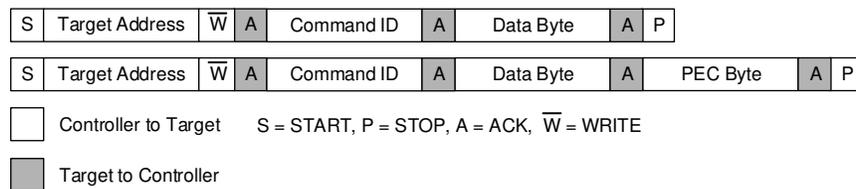
**Figure 8-12. Write Byte**
