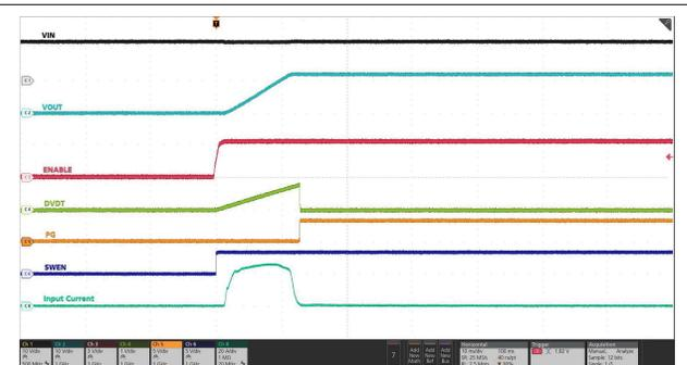
IN supply held steady at 12 V, EN pin toggled from low to high.
