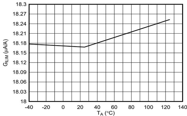
Figure 7-15. ILIM Gain Across Load and Temperature
