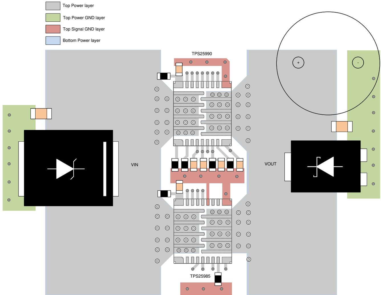
Figure 9-19. TPS25990 and TPS25985x Parallel Devices Layout Example
