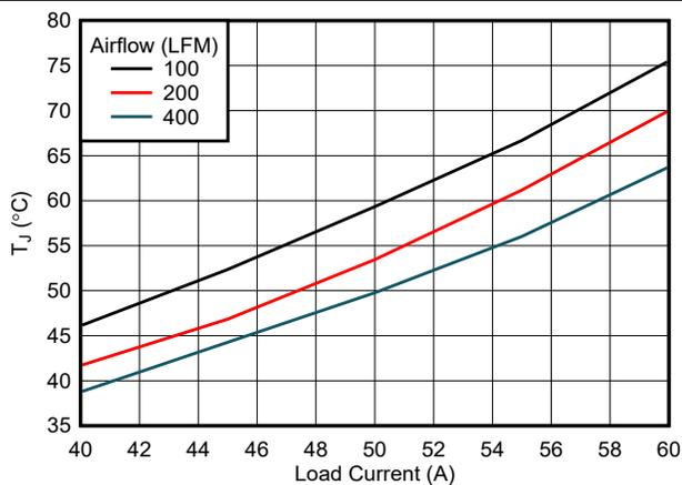
Figure 7-33. Junction Temperature vs Load Current (With Air-Flow)
