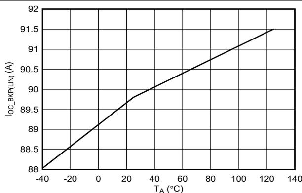
Figure 7-21. Backup Overcurrent Protection Threshold (Steady-state) Accuracy
