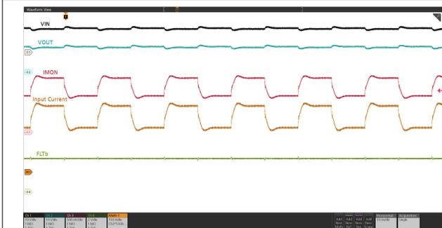
**Figure 9-9. Transient Overload:  $V_{IN} = 12$  V,  $t_{OC\_TIMER} = 10$  ms,  $C_{LOAD} = 50$  mF,  $R_{IMON} = 150 \Omega$ ,  $V_{IREF} = 1$  V, and Load Current Stepped from 333 A to 500 A then 333 A within 8.5 ms**
