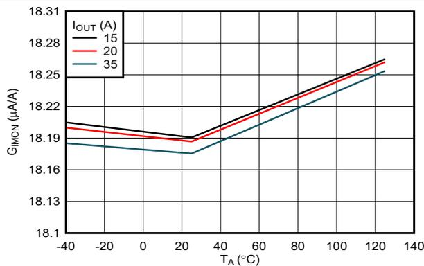
**Figure 7-11. IMON Gain Across Load and Temperature**
