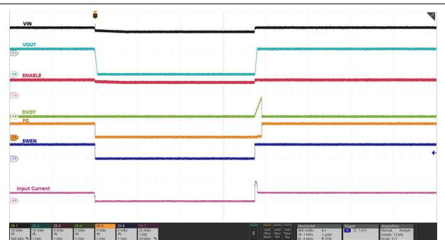
VIN Undervoltage falling threshold programmed to 10.8 V ( $VIN\_UV\_FLT = 0x8D$ ), EN held high, IN supply ramped down from 12 V to 10.5 V and then ramped up again to 12 V.  $C_{OUT} = 18\text{ mF}$ ,  $C_{dVdt} = 33\text{ nF}$
