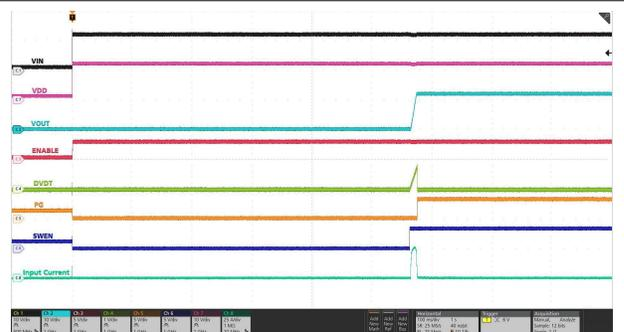
IN hot-plugged to 12 V supply. C<sub>OUT</sub> = 18 mF, C<sub>dVdt</sub> = 33 nF, Insertion Delay programmed to 560 ms (INS\_DLY = 0x07)
