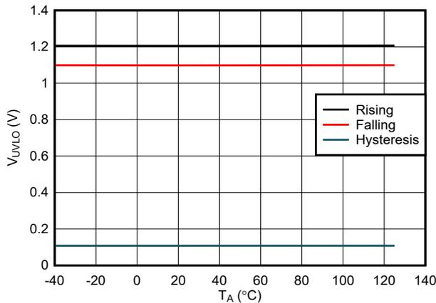
**Figure 7-9. EN/UVLO Based Turn-off Thresholds Across Temperature**
