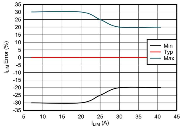
Figure 7-16. Startup Overcurrent Protection Threshold (Current Limit) Accuracy
