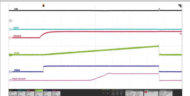
OUT shorted to GND. IN supply held steady at 12 V, EN pin toggled from low to high.
