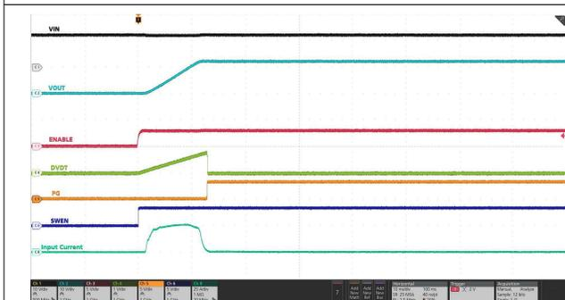
IN supply held steady at 12 V, EN toggled from low to high.  $C_{OUT} = 18\text{ mF}$ ,  $C_{dVdt} = 33\text{ nF}$ , DVDT scaling at 100 % (default),  $DEVICE\_CONFIG[10:9] = 10b$
