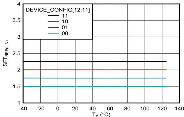
Figure 7-17. Scalable Fast-trip Threshold Ratio Across Temperature (Steady-state)
