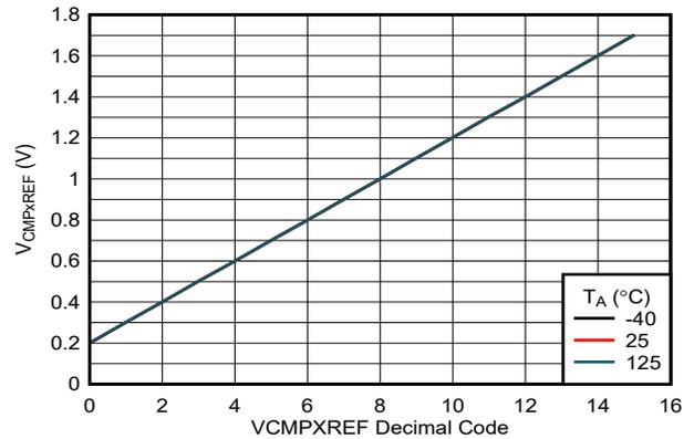
Figure 7-28. General Purpose Comparators Reference DAC Transfer Function
