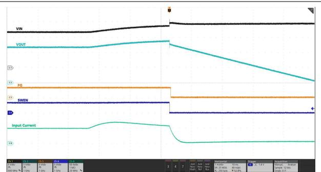
VIN Overvoltage rising threshold programmed to 13.78 V ( $VIN\_OV\_FLT = 0x0B$ ), EN held high, IN supply ramped up from 12 V to 15 V and then ramped down again to 12 V.  $C_{OUT} = 18\text{ mF}$ ,  $C_{dVdt} = 33\text{ nF}$
