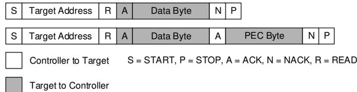
**Figure 8-11. Receive Byte**
