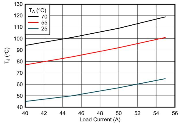
Figure 7-32. Junction Temperature vs Load Current (No Air-Flow)
