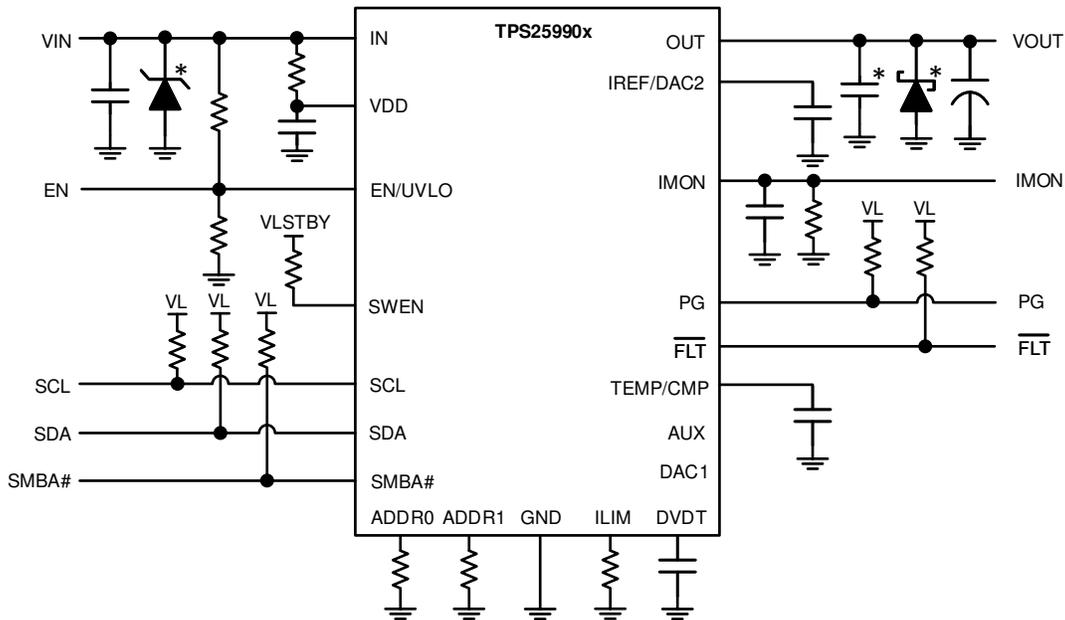
**Figure 9-18. Circuit Implementation with Optional Protection Components**
