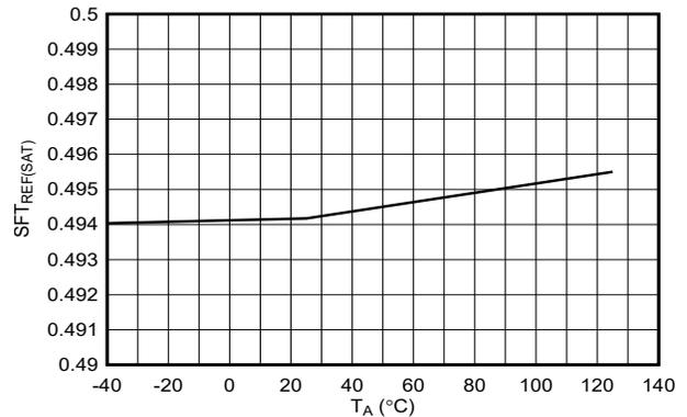
Figure 7-18. Scalable Fast-trip Threshold Ratio Across Temperature (Startup)
