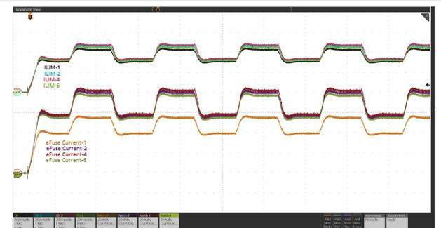
**Figure 9-10. Transient Overload (Current distribution among six devices in parallel):  $V_{IN} = 12$  V,  $t_{OC\_TIMER} = 10$  ms,  $C_{LOAD} = 50$  mF,  $R_{IMON} = 150 \Omega$ ,  $V_{IREF} = 1$  V, and Load Current Stepped from 333 A to 500 A then 333 A within 8.5 ms**
