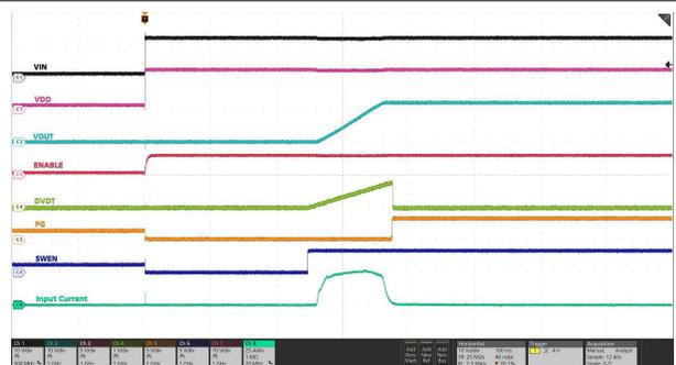
IN hot-plugged to 12 V supply. C<sub>OUT</sub> = 18 mF, C<sub>dVdt</sub> = 33 nF, Insertion Delay programmed to 25 ms (INS\_DLY = 0x01)
