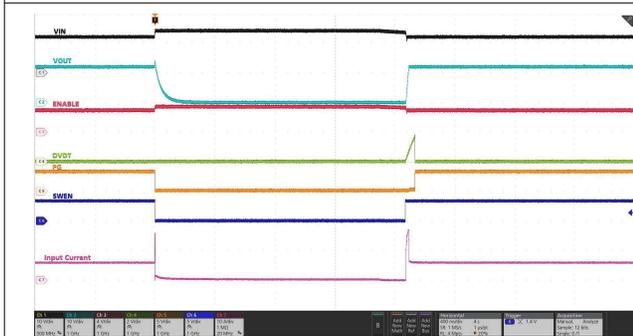
VIN Overvoltage rising threshold programmed to 13.78 V ( $VIN\_OV\_FLT = 0x0B$ ), EN held high, IN supply ramped up from 12 V to 15 V and then ramped down again to 12 V.  $C_{OUT} = 18\text{ mF}$ ,  $C_{dVdt} = 33\text{ nF}$
