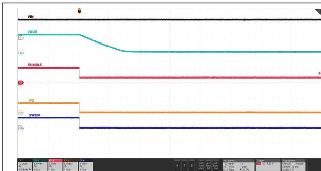
IN supply held steady at 12 V, EN pin pulled down to 1 V for > 5 ms.  $C_{OUT} = 18\text{ mF}$ ,  $C_{dVdt} = 33\text{ nF}$ ,  $I_{LOAD} = 0\text{ A}$
