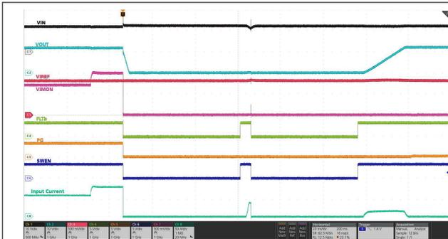
Device in steady-state, Load current ramped up from 50 A to 70 A for 100 ms and then ramped down to 0 A. OCP threshold set to 55 A, Overcurrent blanking delay set to 15 ms (OC\_TIMER = 0x89), Auto-retry 4 times configuration (RETRY\_CONFIG[5:3] = 010b), Auto-retry delay set to 55 ms (RETRY\_CONFIG[2:0] = 000b)
