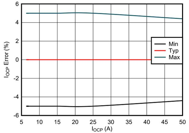
Figure 7-14. Steady-state Overcurrent Protection Threshold (Circuit-Breaker) Accuracy
