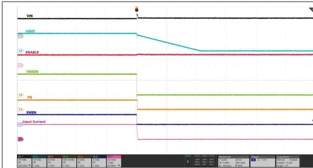
IN supply held steady at 12 V, EN pin held high, PMBus
