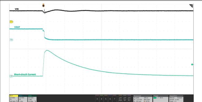
Device in steady-state, OUT shorted to GND. OCP threshold set to 55 A, Short-circuit fast recovery disabled (Default, DEVICE\_CONFIG[13] = 0b)
