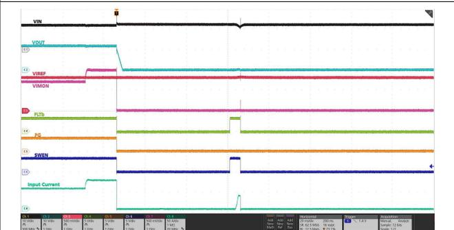
Device in steady-state, Load current ramped up from 50 A to 70 A for 100 ms. OCP threshold set to 55 A, Overcurrent blanking delay set to 15 ms (OC\_TIMER = 0x89), Auto-retry 1 times configuration (RETRY\_CONFIG[5:3] = 001b), Auto-retry delay set to 55 ms (RETRY\_CONFIG[2:0] = 000b)
