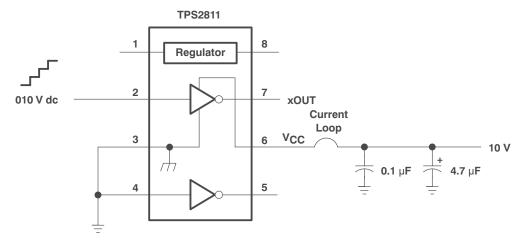
Figure 2. Shoot-Through Current Test Setup
