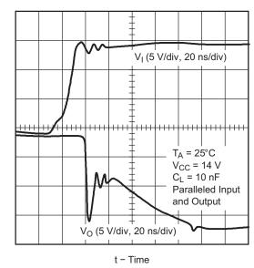
Figure 31. Input Voltage vs Output Voltage, High-to-Low Propagation Delay of Paralleled Drivers
