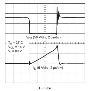
Figure 39. Drain-Source Voltage vs Drain Current, TPS2811 Driving an IRF530 (Hex-3 Size)
