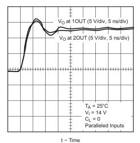
Figure 21. Voltage of 10UT vs Voltage at 20UT, Low-to-High Output Delay
