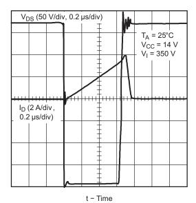
Figure 41. Drain-Source Voltage vs Drain Current, One Driver, TPS2811 Driving an IRF840 (Hex-4 Size)
