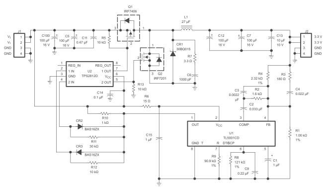
NOTE: If the parasitics of the external circuit cause the voltage to violate the Absolute Maximum Rating for the Output pins, Schottky diodes should be added from ground to output and from output to V<sub>CC</sub>.
