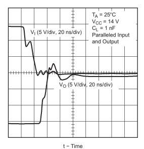
Figure 28. Input Voltage vs Output Voltage, Low-to-High Propagation Delay of Paralleled Drivers
