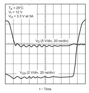
Figure 52. Q1 Drain Voltage vs Q2 Gate-Source Voltage
