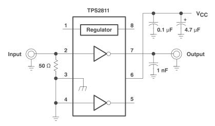
Figure 1. Test Circuit For Measurement of Switching Characteristics
