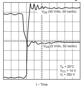
Figure 47. Drain-Source Voltage vs Gate-Source Voltage, at Turn-off, Parallel Drivers, TPS2811 Driving an IRF840 (Hex-4 Size)
