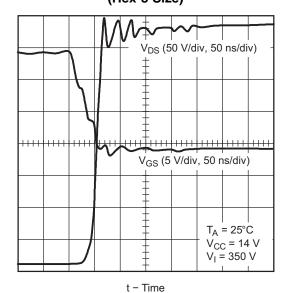
Figure 44. Drain-Source Voltage vs Gate-Source Voltage, at Turn-off, One Driver, TPS2811 Driving an IRF840 (Hex-4 Size)
