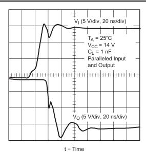
Figure 29. Input Voltage vs Output Voltage, High-to-Low Propagation Delay of Paralleled Drivers
