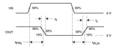
Figure 3. Typical Timing Diagram
