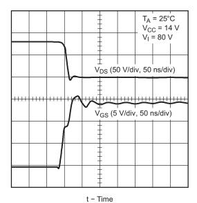
Figure 37. Drain-Source Voltage vs Gate-Source Voltage, at Turn-on, TPS2811 Driving an IRFD120 (Hex-2 Size)
