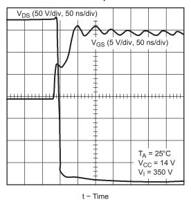
Figure 43. Drain-Source Voltage vs Gate-Source Voltage, at Turn-on, One Driver, TPS2811 Driving an IRF840 (Hex-4 Size)
