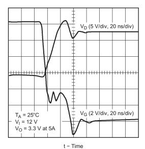
Figure 49. Q1 Drain Voltage vs Gate Voltage, at Switch Turn-on
