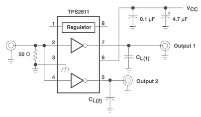
A. Input rise and fall times should be ≤10 ns for accurate measurement of ac parameters.
