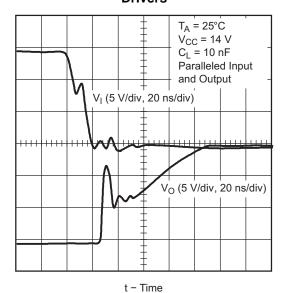
Figure 30. Input Voltage vs Output Voltage, Low-to-High Propagation Delay of Paralleled Drivers
