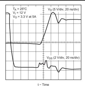
Figure 53. Q1 Drain Voltage vs Q2 Gate-Source Voltage
