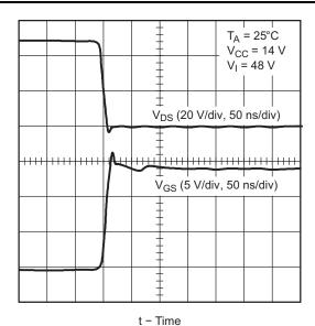
Figure 34. Drain-Source Voltage vs Gate-Source Voltage, at Turn-on, TPS2811 Driving an IRFD014
