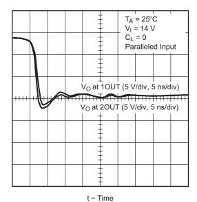
Figure 22. Voltage at 10UT vs Voltage at 20UT, High-to-Low Output Delay
