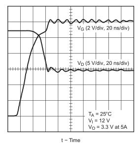
Figure 50. Q1 Drain Voltage vs Gate Voltage, at Switch Turn-off
