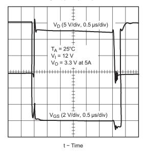
Figure 51. Q1 Drain Voltage vs Q2 Gate-Source Voltage
