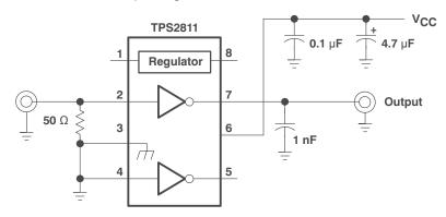
Figure 19. Test Circuit for Measuring Switching Characteristics
