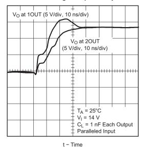
Figure 23. Voltage at 10UT vs Voltage at 20UT, Low-to-High Output Delay
