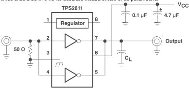
Figure 27. Test Circuit for Measuring Paralleled Switching Characteristics
