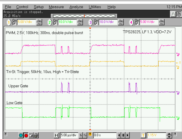
Figure 7-3. 2.5-V Amplitude PWM Pulse (TPS28225-Q1)
