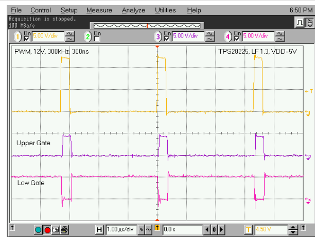
Figure 7-5. 12-V PWM Pulse at V_{DD} = 5 V
